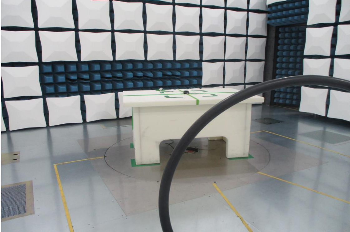
Figure 17: 9kHz-30MHz Test Setup (Front View)
