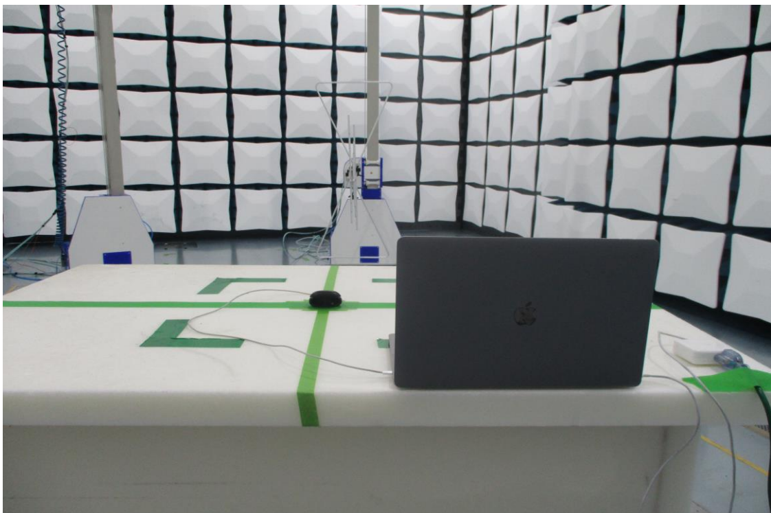
Figure 12: 30MHz-1GHz Test Setup (Rear View)
