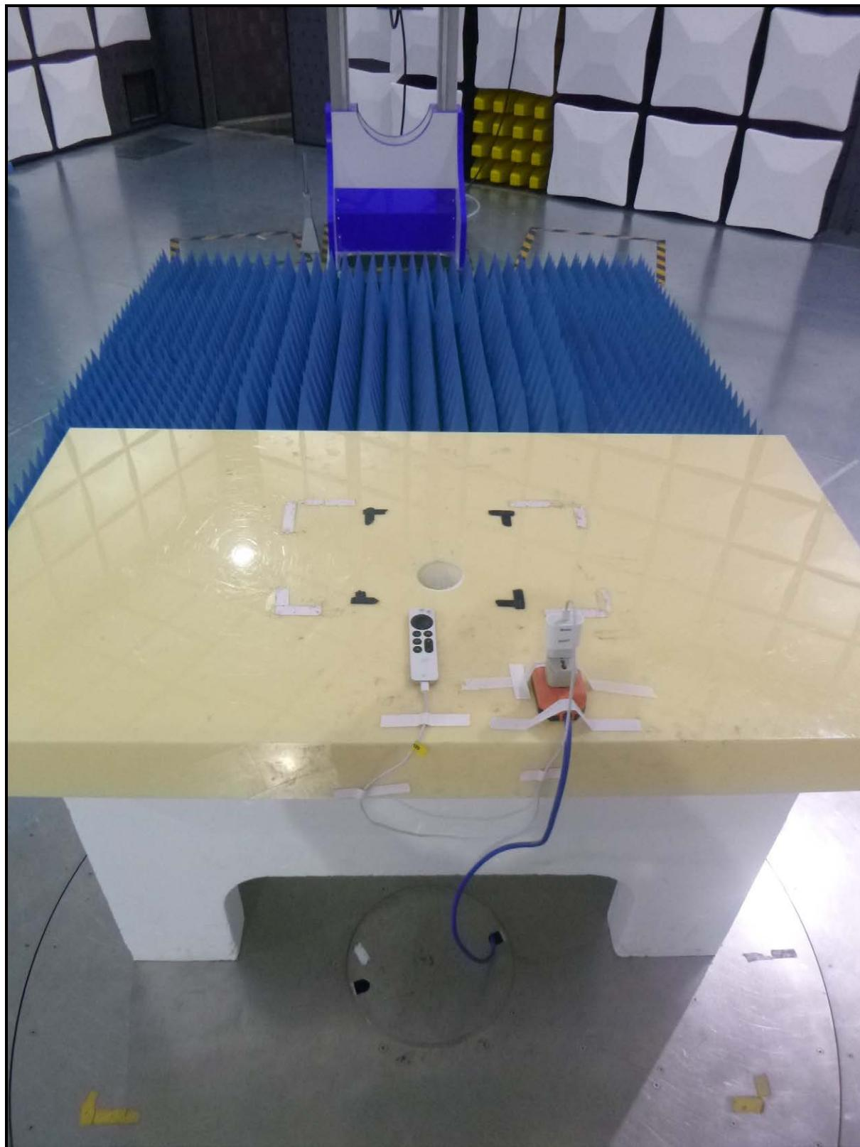
PHT\14247018JD18\002 - Test Configuration Photograph - Radiated Emissions 002
