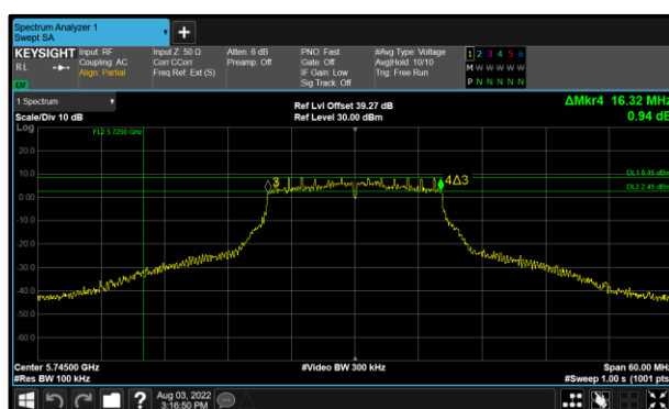
Figure 85 - 802.11a Minimum 6 dB EBW
