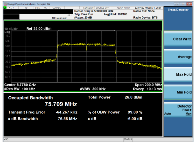
Plot 7-250. 6dB BW & 99% OBW Antenna 2a (80MHz BW 802.11ac – Ch. 155, MCS9)
