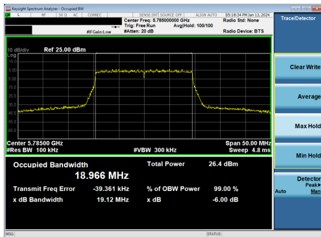
Plot 7-223. 6dB BW & 99% OBW Antenna 4a (20MHz BW 802.11ax(SU) – Ch. 157, MCS4)
