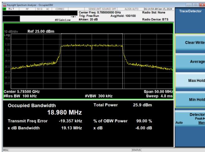
Plot 7-211. 6dB BW & 99% OBW Antenna WF5b (20MHz BW 802.11ax(SU) – Ch. 157, MCS11)
