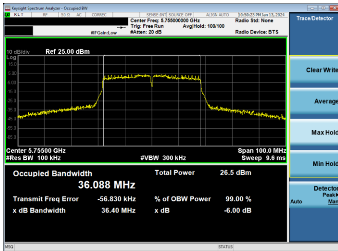
Plot 7-242. 6dB BW & 99% OBW Antenna 2a (40MHz BW 802.11n – Ch. 151, MCS4)
