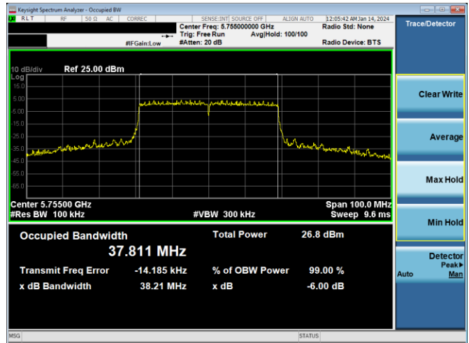
Plot 7-249. 6dB BW & 99% OBW Antenna 2a (40MHz BW 802.11ax(SU) – Ch. 151, MCS11)
