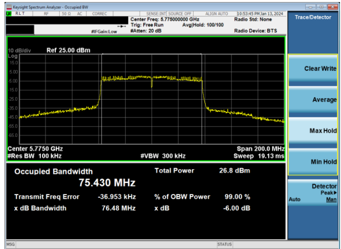
Plot 7-244. 6dB BW & 99% OBW Antenna 2a (80MHz BW 802.11ac – Ch. 155, MCS4)
