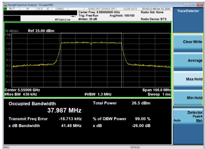
Plot 7-18. 26dB BW & 99% OBW Antenna WF5b (40MHz BW 802.11ax(SU) – Ch. 110, MCS2)
