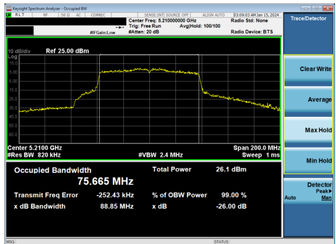
Plot 7-5. 26dB BW & 99% OBW Antenna WF5b (80MHz BW 802.11ac – Ch. 42, MCS2)
