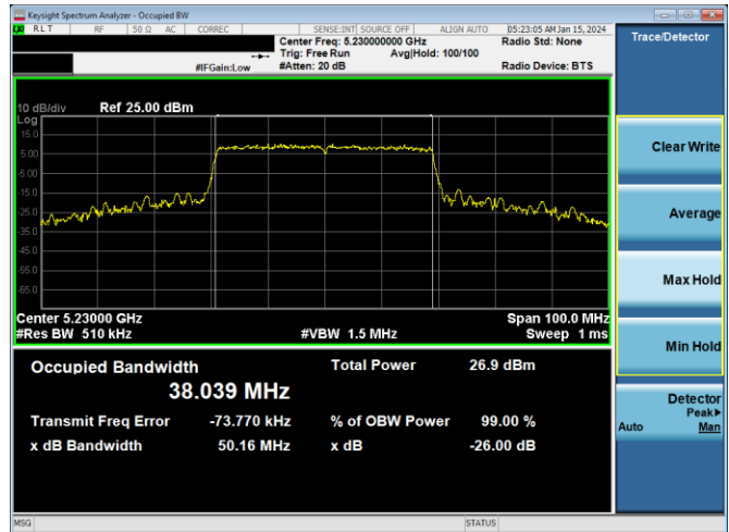
Plot 7-48. 26dB BW & 99% OBW Antenna WF5b (40MHz BW 802.11ax(SU) – Ch. 46, MCS11)
