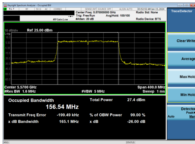
Plot 7-22. 26dB BW & 99% OBW Antenna WF5b (160MHz BW 802.11ac - Ch. 114, MCS2)
