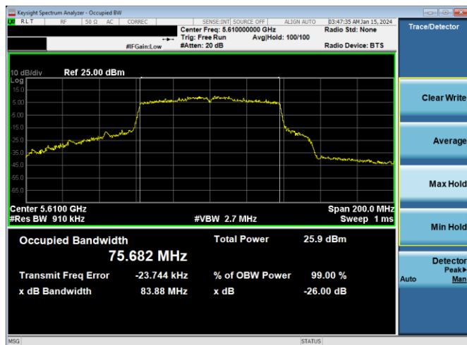
Plot 7-19. 26dB BW & 99% OBW Antenna WF5b (80MHz BW 802.11ac - Ch. 122, MCS2)
