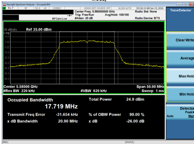
Plot 7-15. 26dB BW & 99% OBW Antenna WF5b (20MHz BW 802.11n – Ch. 116, MCS2)
