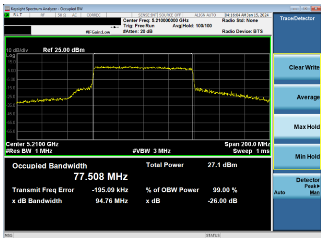
Plot 7-28. 26dB BW & 99% OBW Antenna WF5b (80MHz BW 802.11ax(SU) – Ch. 42, MCS4)
