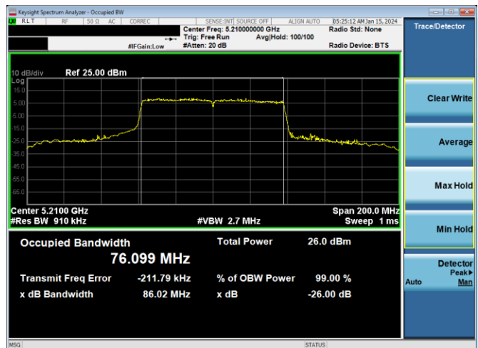
Plot 7-49. 26dB BW & 99% OBW Antenna WF5b (80MHz BW 802.11ac – Ch. 42, MCS9)
