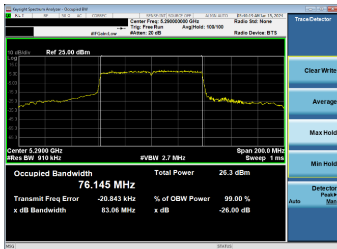
Plot 7-57. 26dB BW & 99% OBW Antenna WF5b (80MHz BW 802.11ac – Ch. 58, MCS9)
