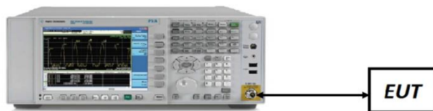
Figure 7-1. Test Instrument & Measurement Setup
