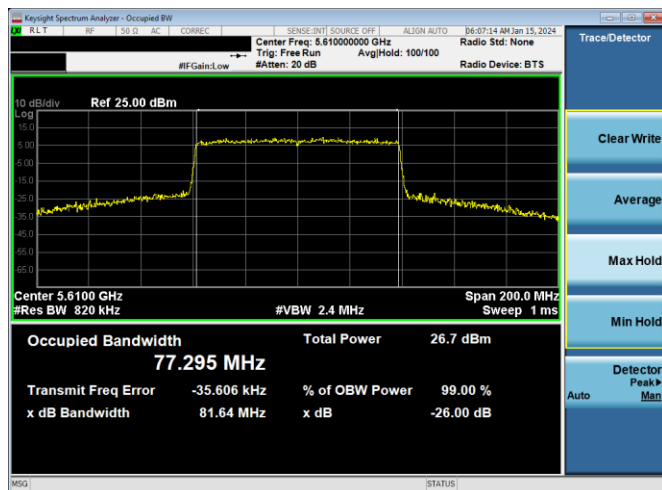
Plot 7-64. 26dB BW & 99% OBW Antenna WF5b (80MHz BW 802.11ax(SU) – Ch. 122, MCS11)
