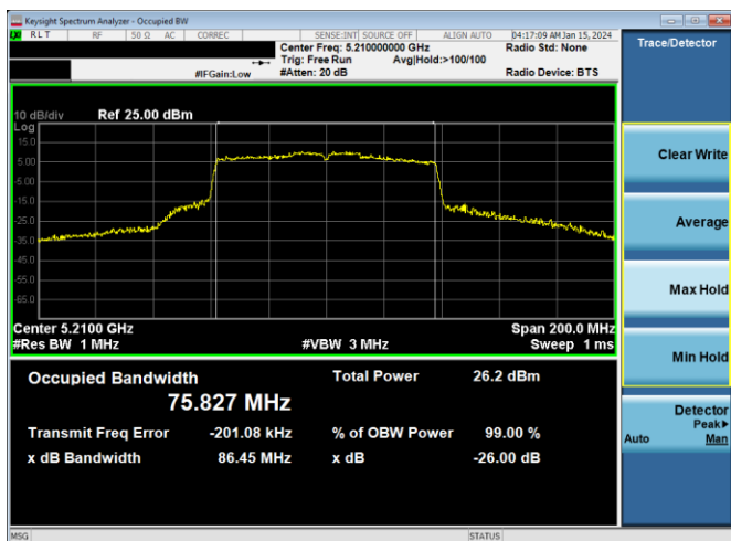
Plot 7-27. 26dB BW & 99% OBW Antenna WF5b (80MHz BW 802.11ac – Ch. 42, MCS4)
