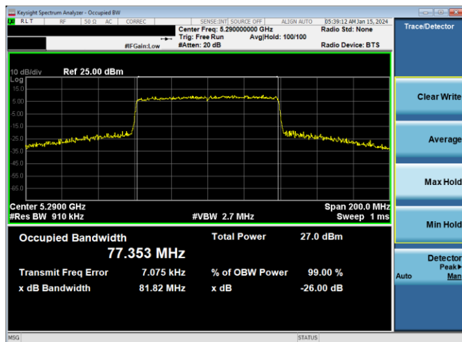
Plot 7-58. 26dB BW & 99% OBW Antenna WF5b (80MHz BW 802.11ax(SU) – Ch. 58, MCS11)
