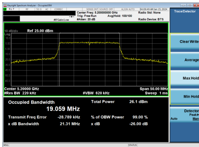
Plot 7-24. 26dB BW & 99% OBW Antenna WF5b (20MHz BW 802.11ax(SU) – Ch. 40, MCS4)
