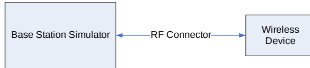
Figure 8-1 Power Measurement Setup
