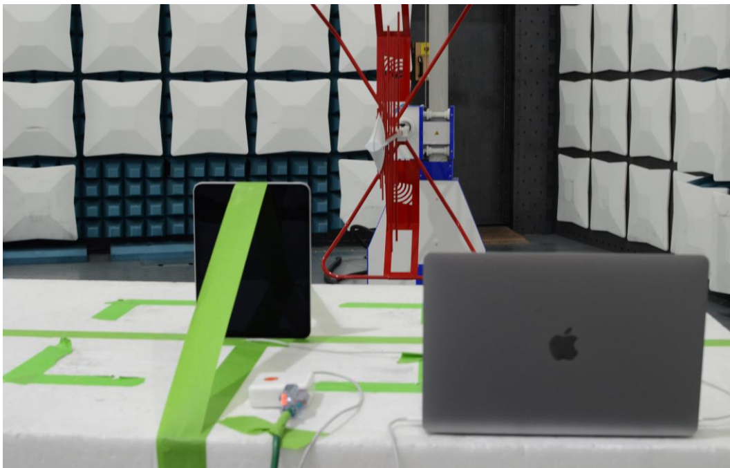
Figure 22: 30MHz-1GHz Test Setup (Rear View)
