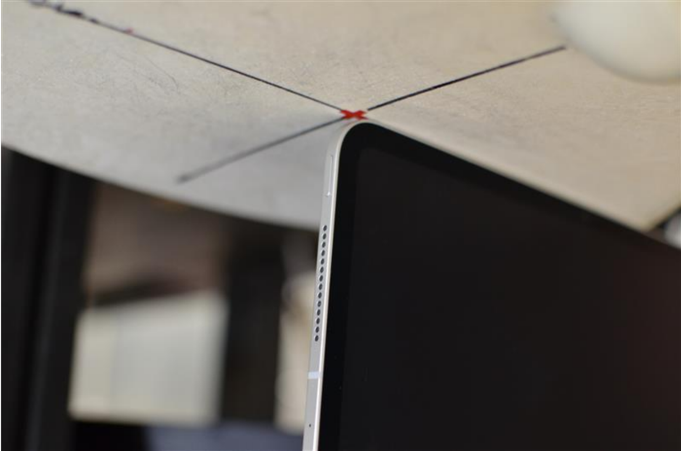
SAR Test Setup Photo 6: Body, Right Edge at 0.0 cm – Antenna 3/4a/4b
