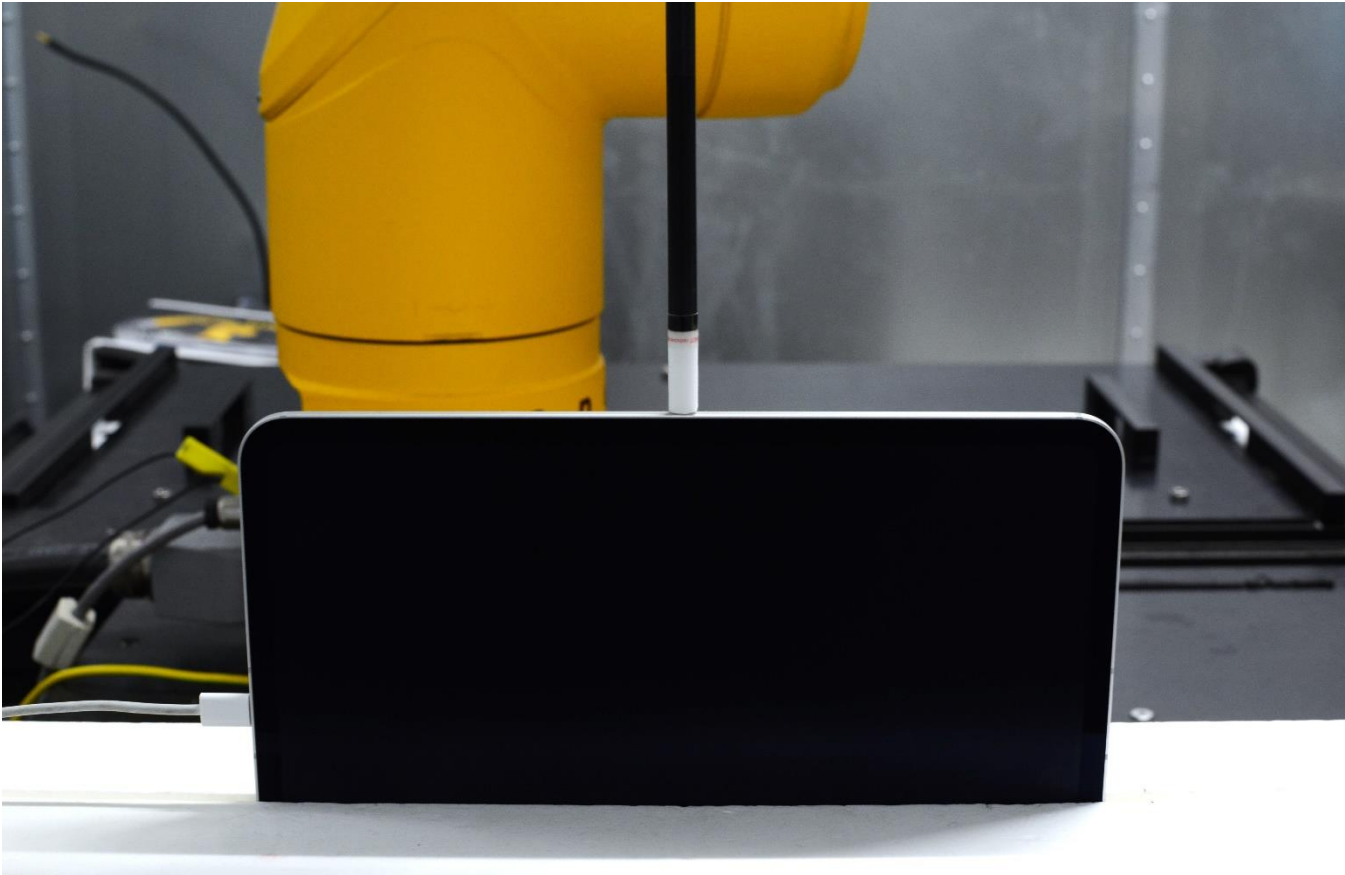
Near Field Power Density Test Setup 19: Left Edge at 2mm
