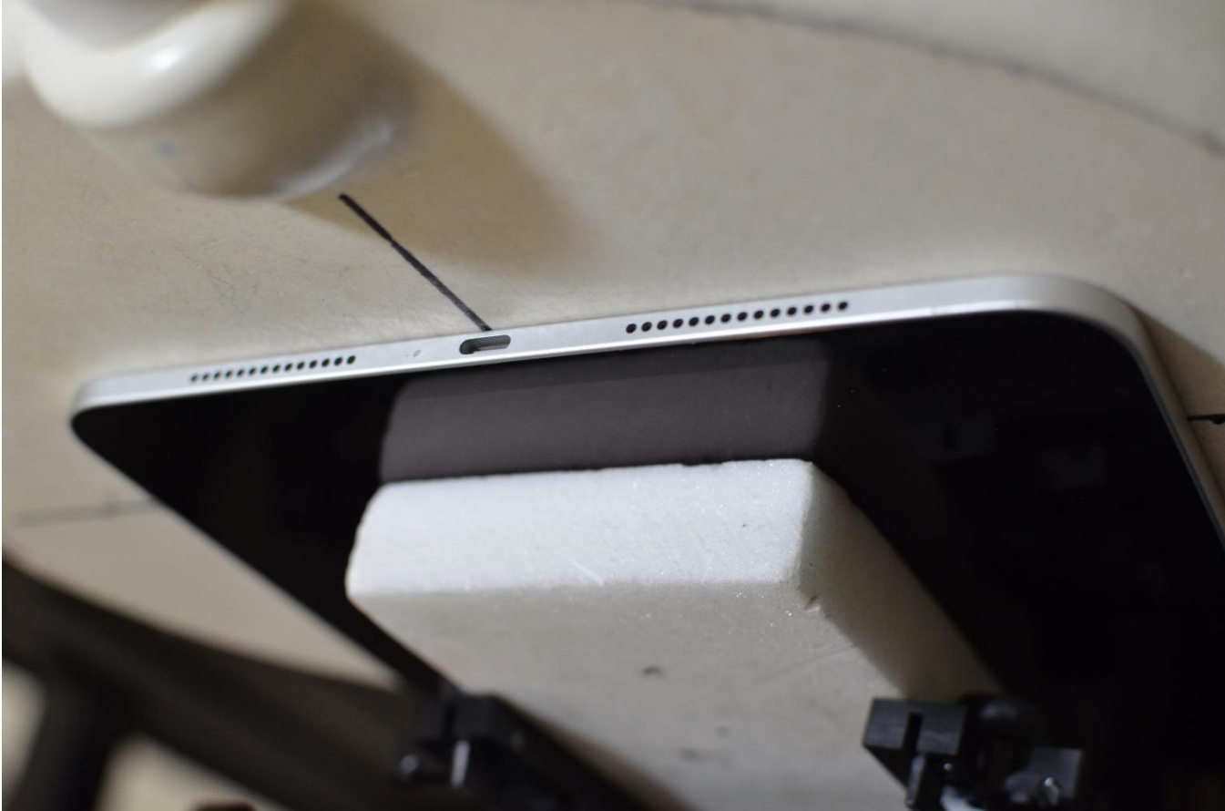
SAR Test Setup Photo 1: Body, Back Side at 0.0 cm – Antenna 1/2a/2b/WF5B
