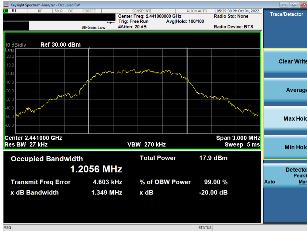
Plot 7-5. 20dB BW and 99% OBW Plot (Bluetooth, 8DPSK, ePA – Ch. 39)
