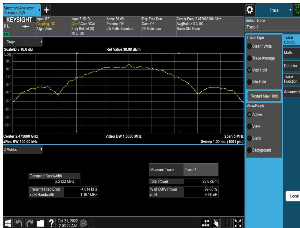
Plot 7-3. 6dB BW & 99% OBW Plot (802.15.4, Ch. 25)
