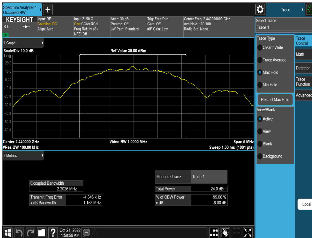
Plot 7-2. 6dB BW & 99% OBW Plot (802.15.4, Ch. 18)
