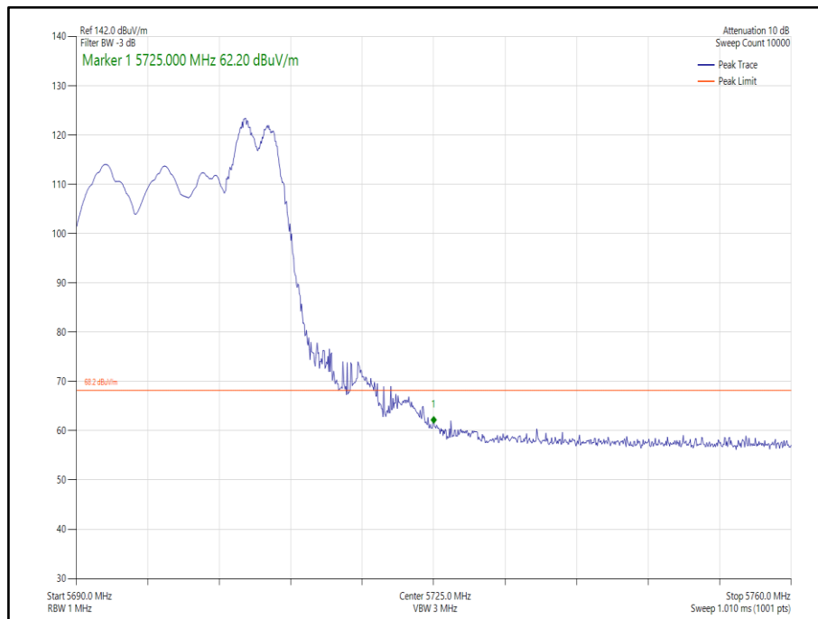
Figure 239 - 802.11ax HE20 SDM, Cores 0-1, 52-40 - 5700 MHz, Band Edge Frequency 5725 MHz
