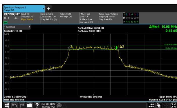
Figure 160 - 802.11n HT20 Minimum 6 dB EBW
