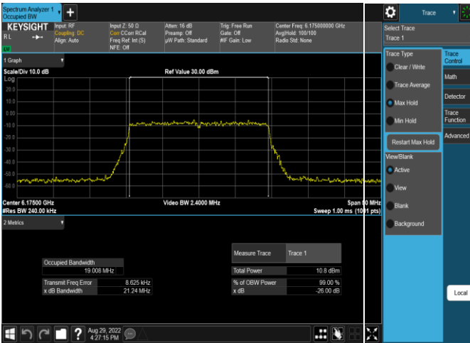
Plot 7-102. 26dB & 99% Bandwidth Plot Antenna 4a (20MHz 802.11ax (UNII Band 5) – Ch. 45, MCS11)
