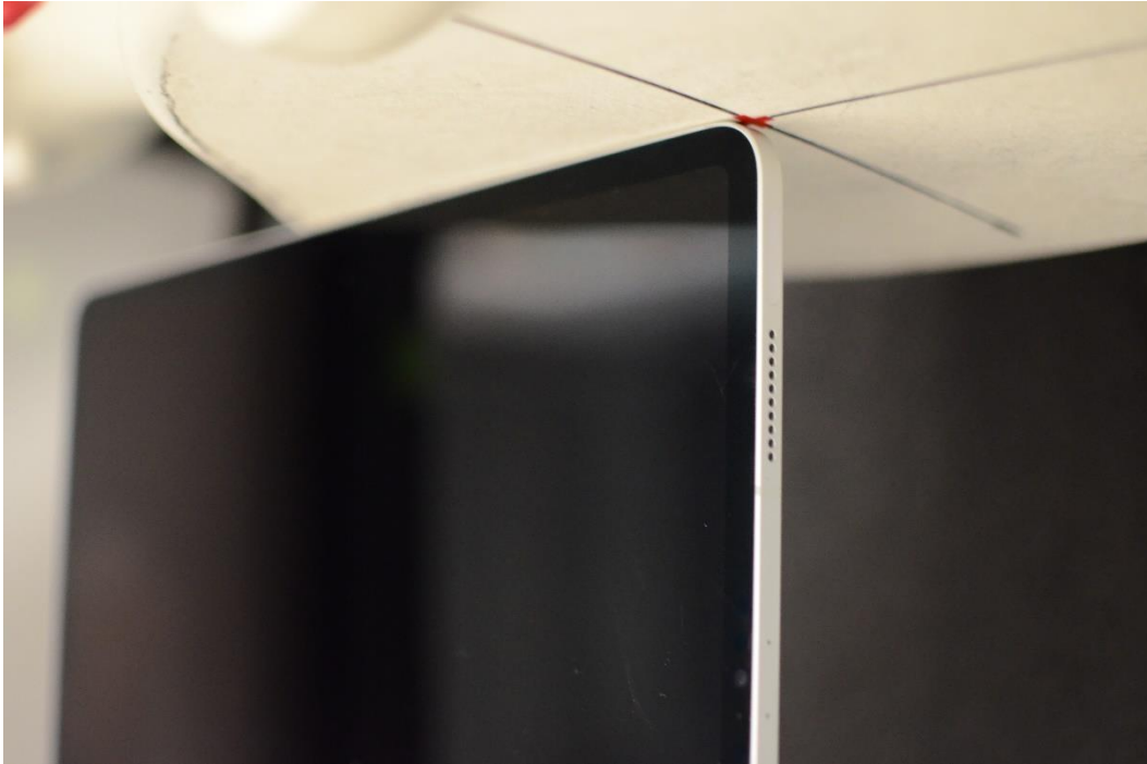
Figure G-9 SAR Test Setup Photo – Left Edge at 0mm – Antenna 4A
