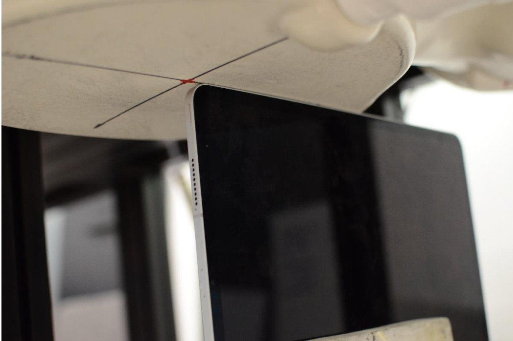
Figure G-7 SAR Test Setup Photo – Right Edge at 0 mm – Antenna 4A
