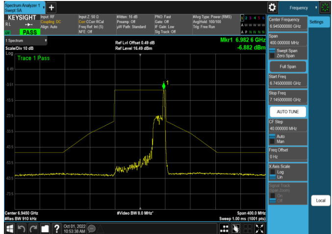
Plot 7-443. In-Band Emission Plot Antenna 5b (80MHz 802.11ax RU26 (UNII Band 8) – Ch. 199)
