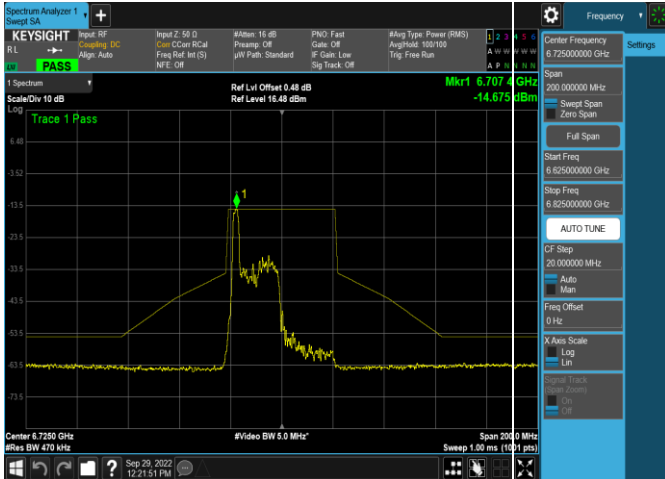
Plot 7-485. In-Band Emission Plot Antenna 4a (40MHz 802.11ax RU26 (UNII Band 7) – Ch. 155)
