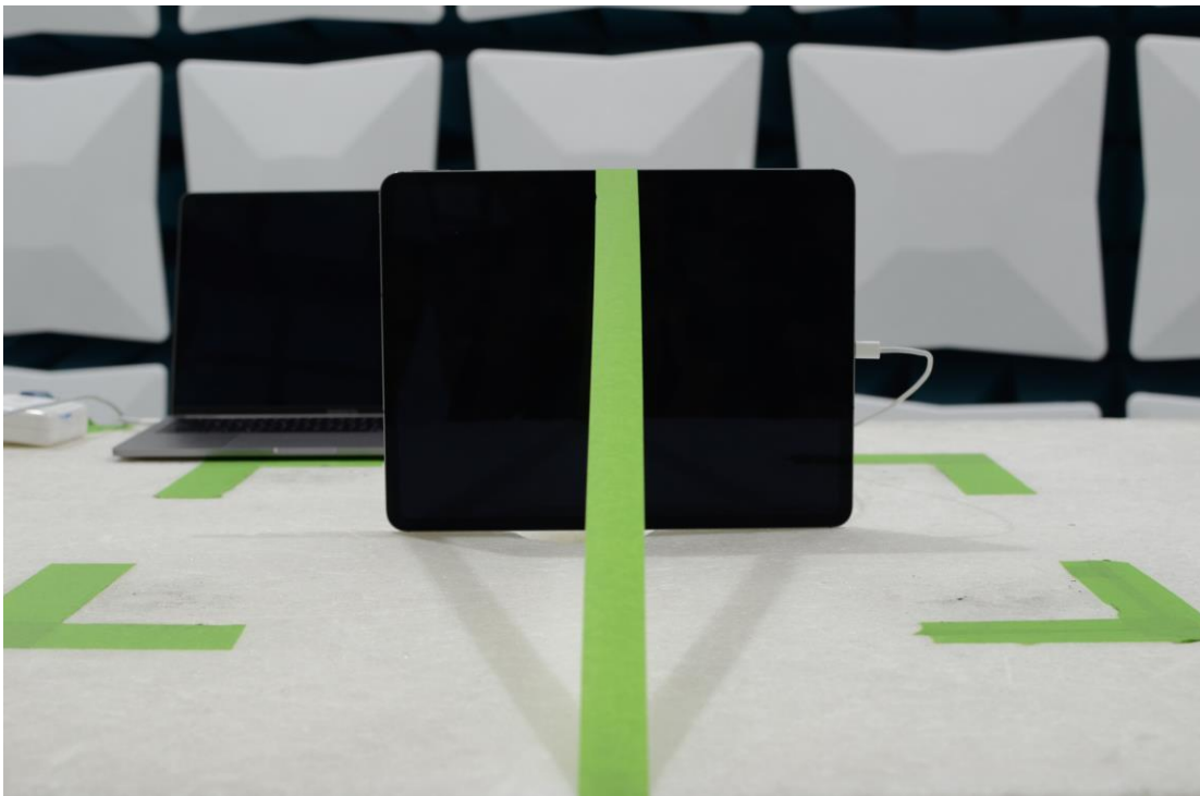
Figure 20: 30MHz-1GHz Test Setup (Front View)
