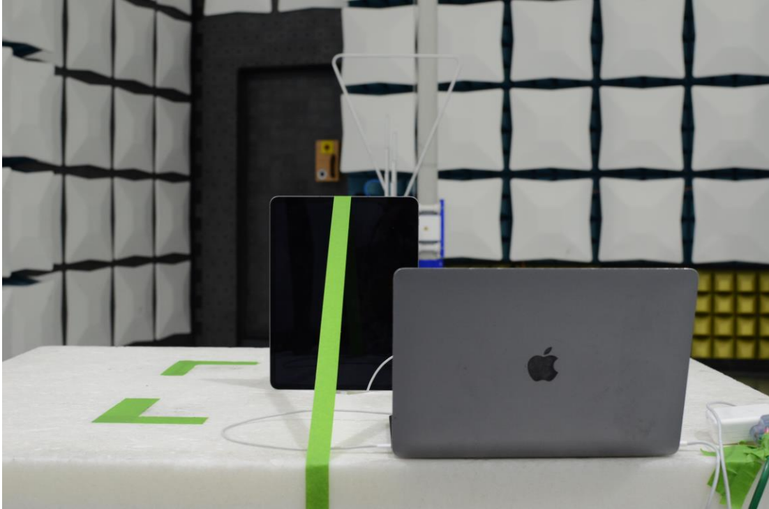
Figure 23: 30MHz-1GHz Test Setup (Rear View)
