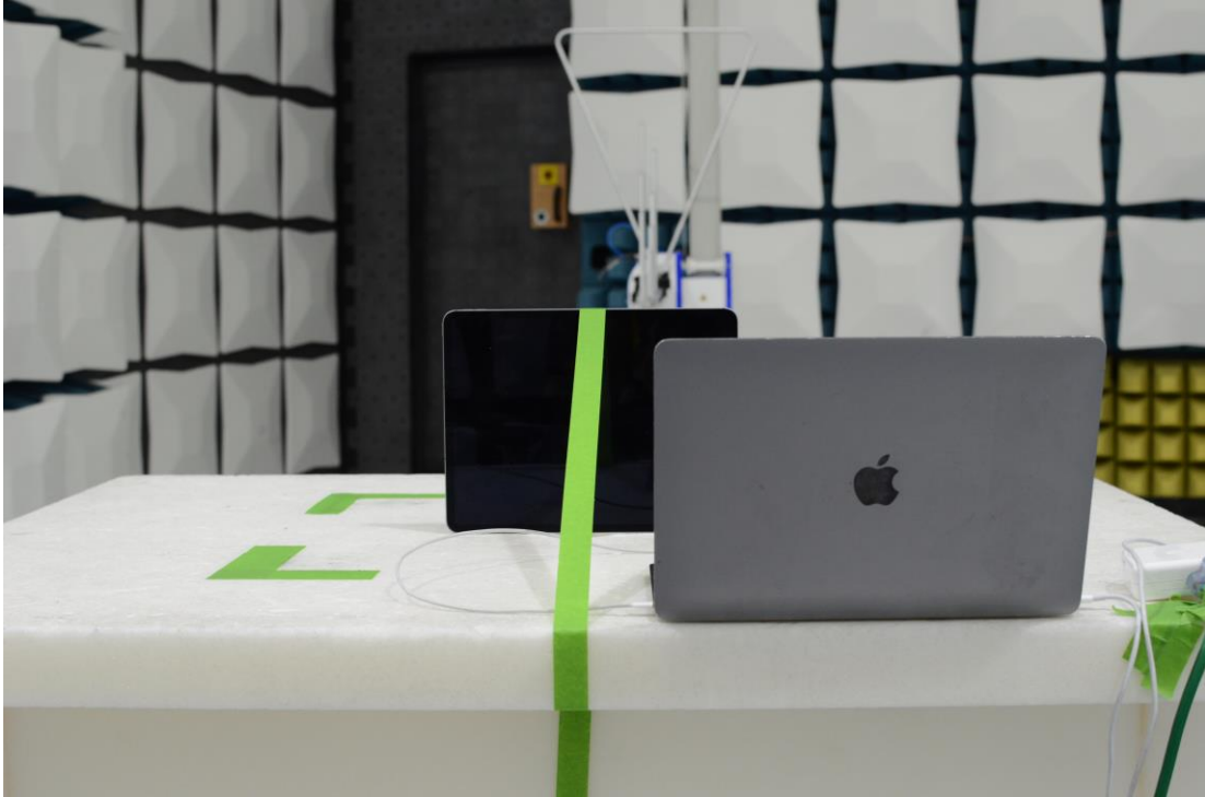
Figure 21: 30MHz-1GHz Test Setup (Rear View)
