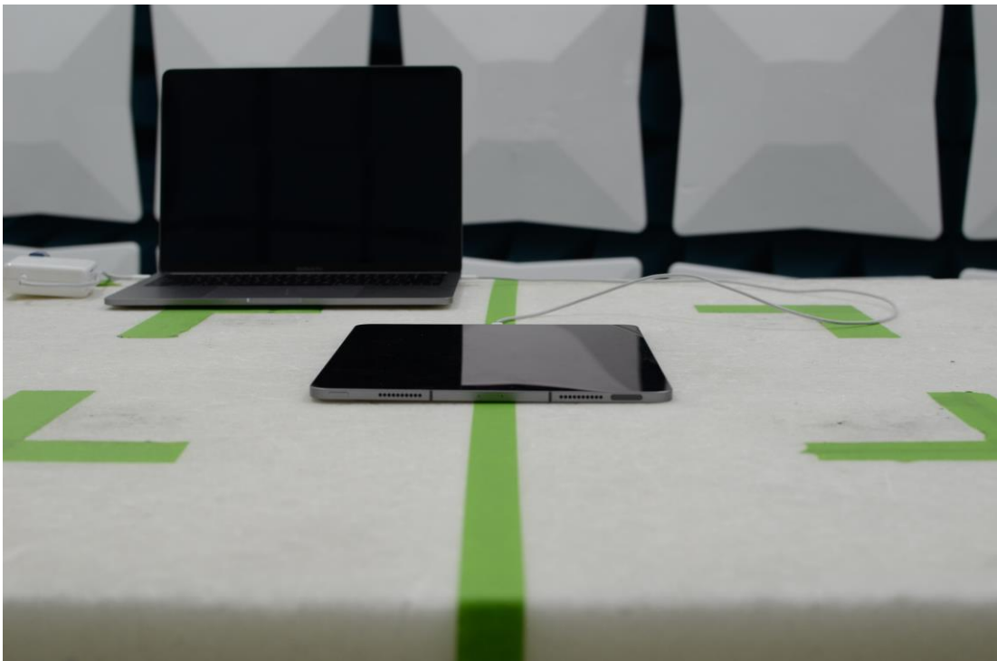
Figure 18: 30MHz-1GHz Test Setup (Front View)
