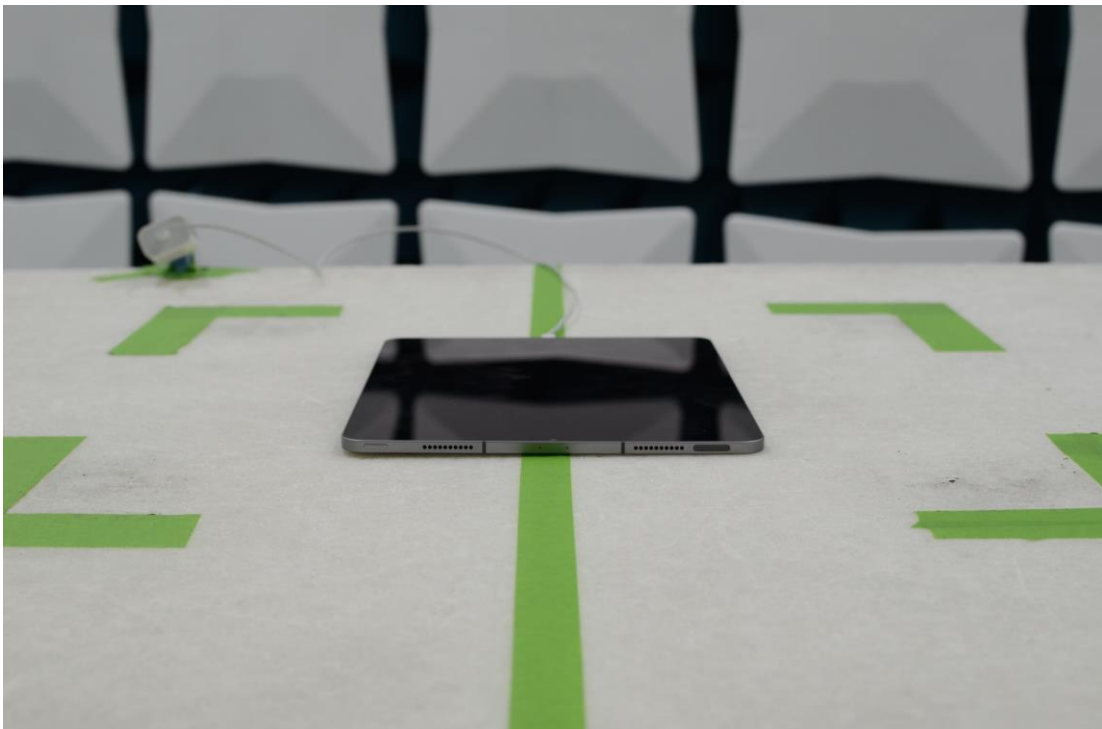
Figure 12: 30MHz-1GHz Test Setup (Front View)
