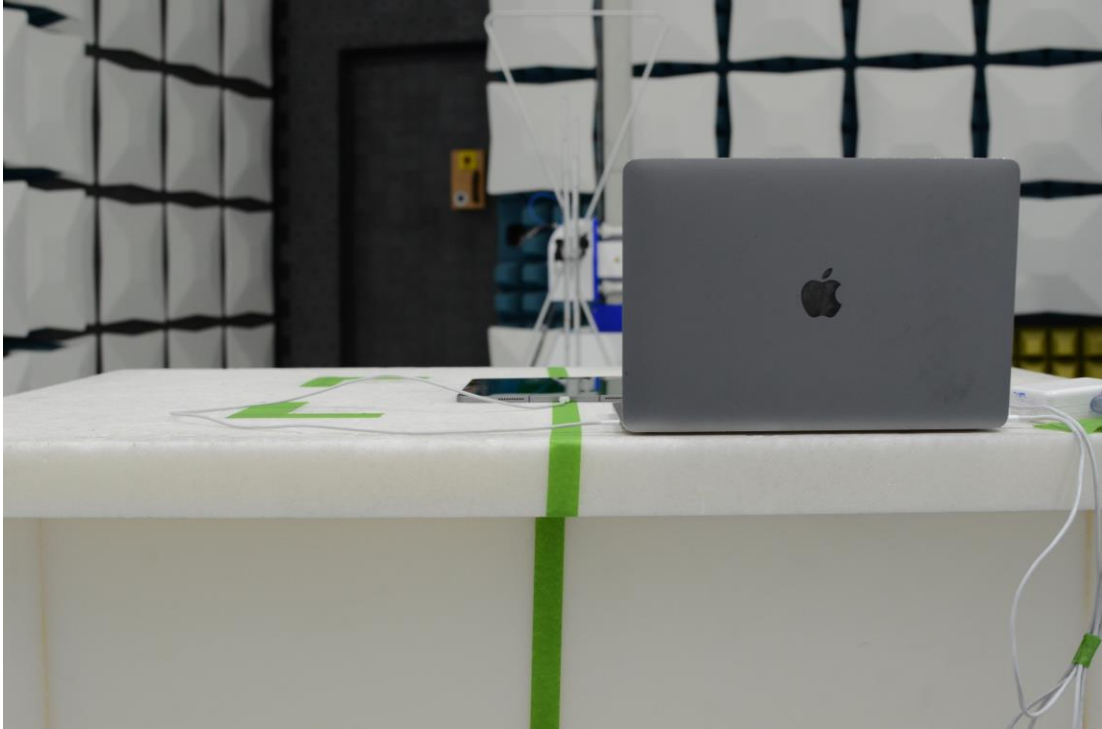
Figure 19: 30MHz-1GHz Test Setup (Rear View)
