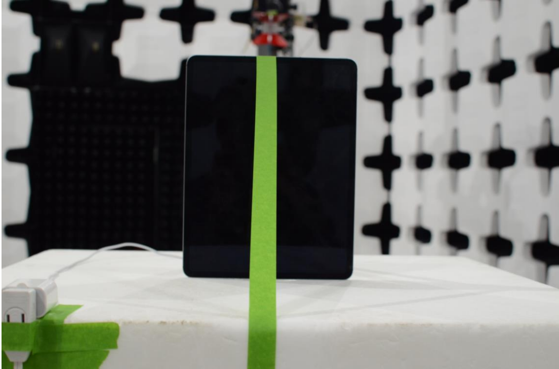
Figure 11: 1-18GHz Test Setup (Rear View)
