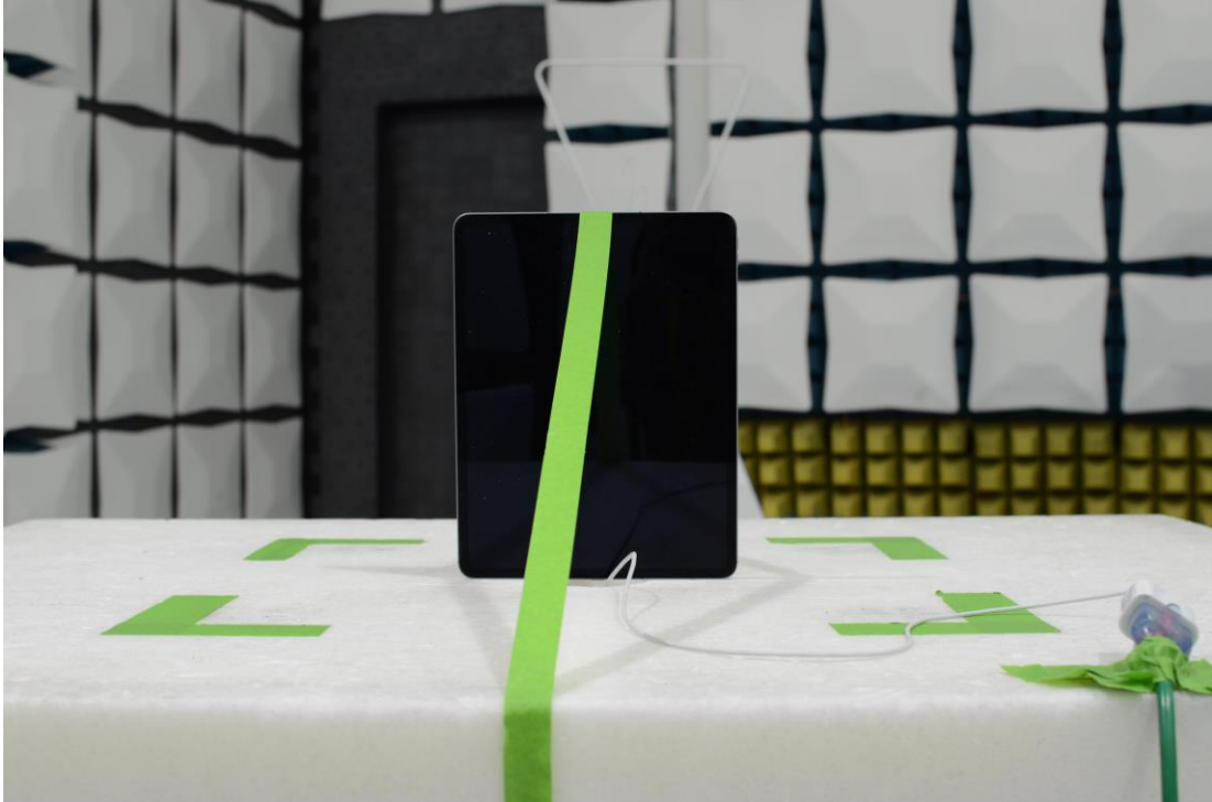
Figure 17: 30MHz-1GHz Test Setup (Rear View)
