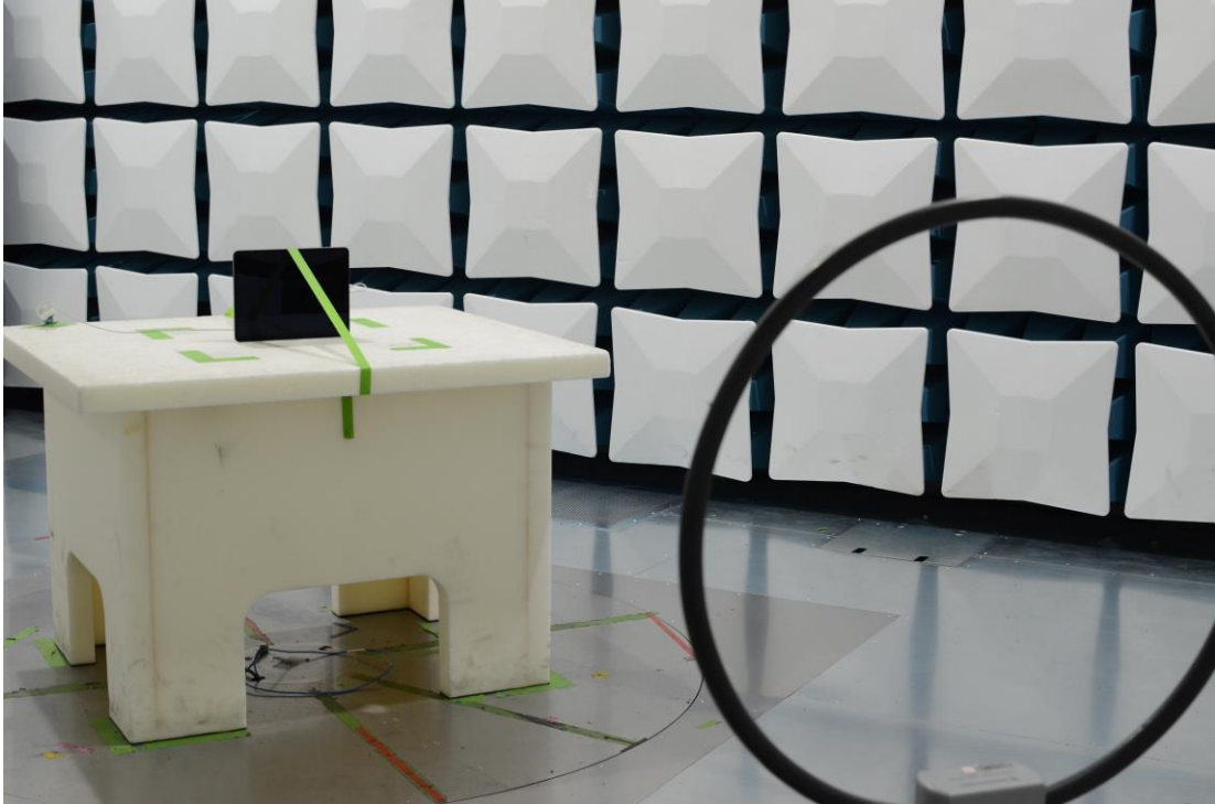
Figure 25: 9kHz-30MHz Test Setup (Front View)
