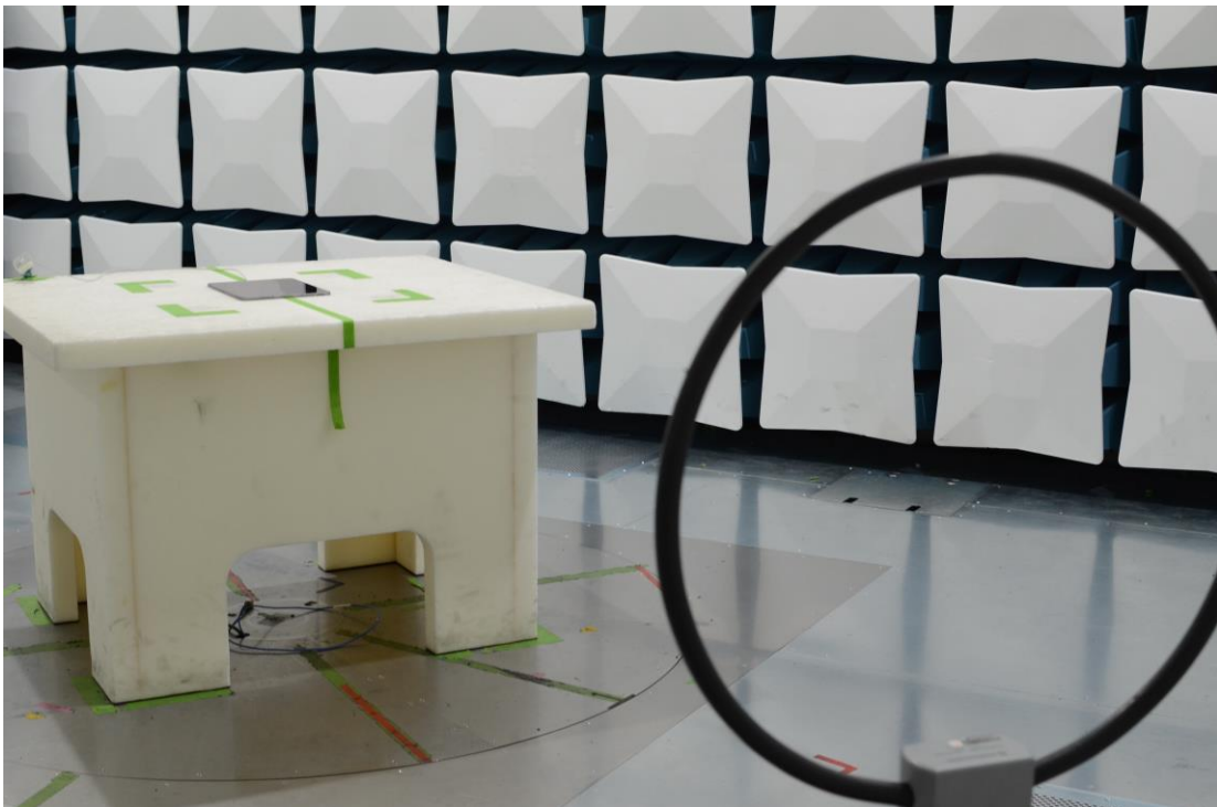
Figure 24: 9kHz-30MHz Test Setup (Front View)
