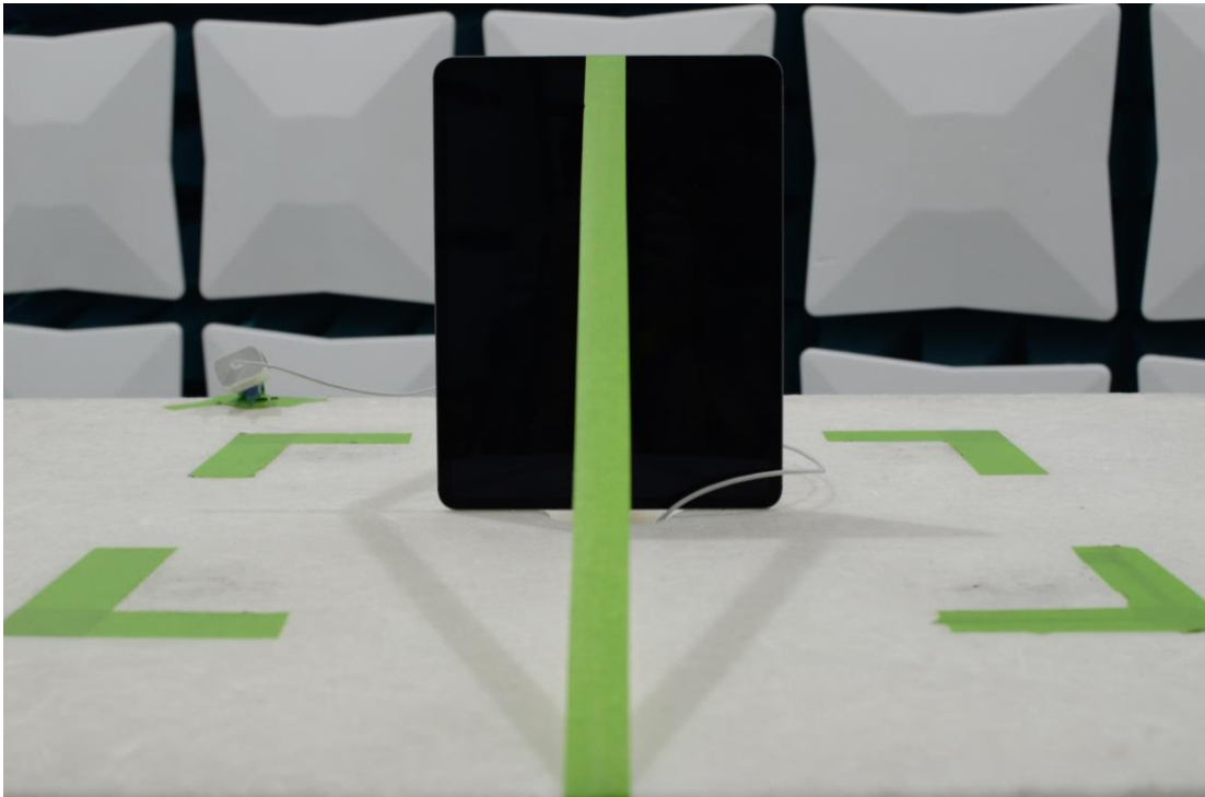
Figure 16: 30MHz-1GHz Test Setup (Front View)
