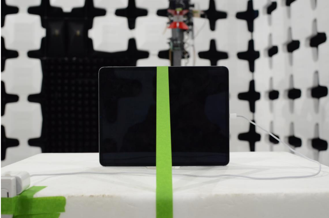
Figure 9: 1-18GHz Test Setup (Rear View)
