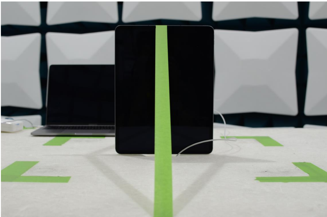
Figure 22: 30MHz-1GHz Test Setup (Front View)
