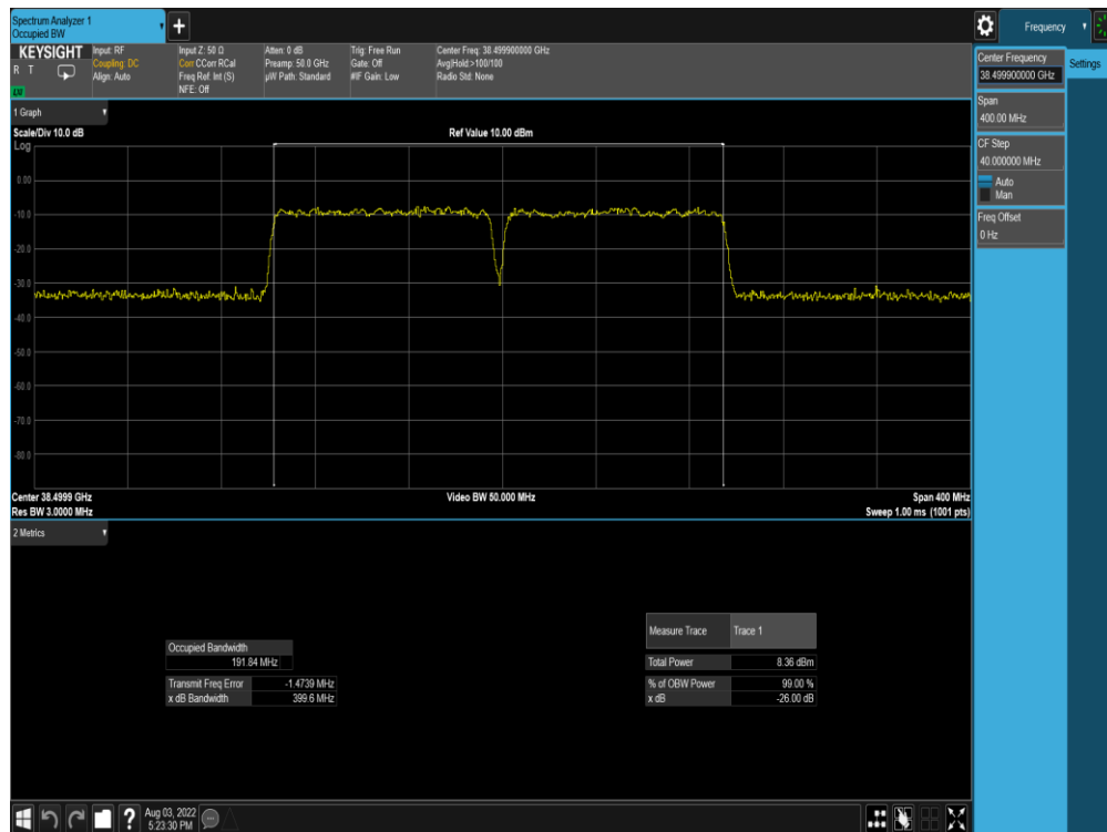
Plot 7-384. Ant M0 OBW (Band n260-100MHz-2CC SISO DFTs-OFDM – 16QAM – Mid Channel)
