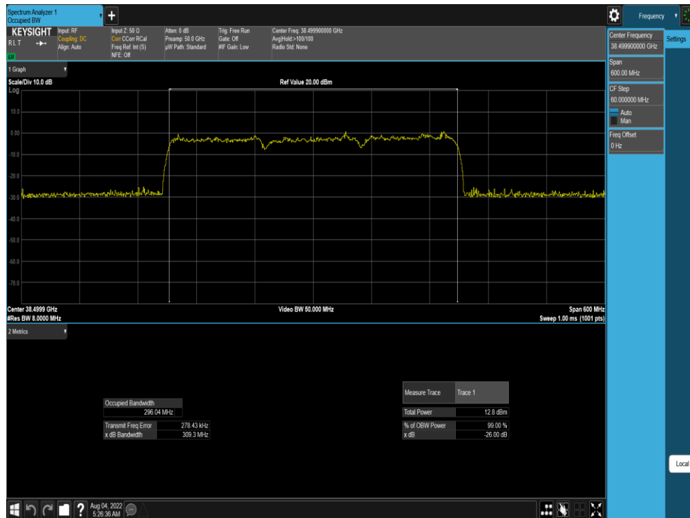
Plot 7-395. Ant M0 OBW (Band n260-100MHz-3CC SISO CP-OFDM – 64QAM – Mid Channel)
