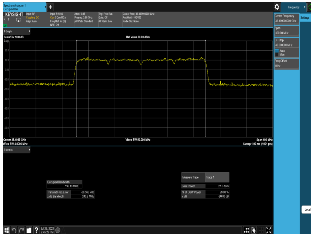
Plot 7-363. Ant M0 OBW (Band n260-50MHz-4CC SISO Dual Pol DFTs-OFDM – 16QAM – Mid Channel)
