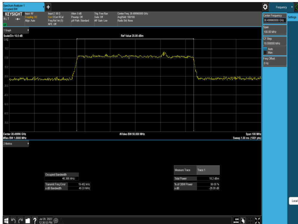
Plot 7-312. Ant M0 OBW (Band n260-50MHz-1CC SISO DFTs-OFDM – \pi/2 BPSK – Mid Channel)
