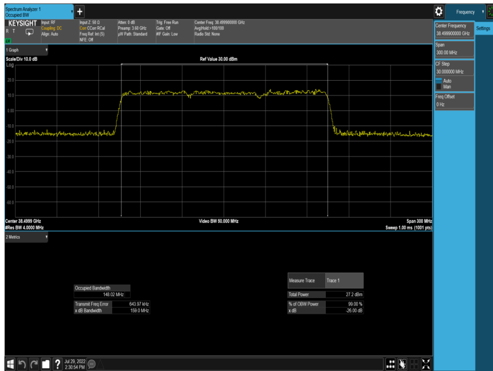
Plot 7-345. Ant M0 OBW (Band n260-50MHz-3CC MIMO CP-OFDM – 16QAM – Mid Channel)
