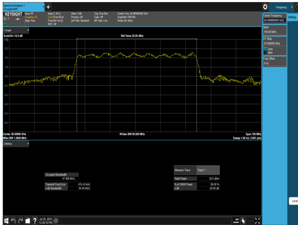
Plot 7-316. Ant M0 OBW (Band n260-50MHz-1CC MIMO CP-OFDM – QPSK – Mid Channel)
