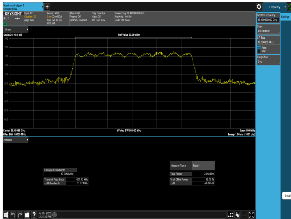
Plot 7-317. Ant M0 OBW (Band n260-50MHz-1CC MIMO CP-OFDM – 16QAM – Mid Channel)
