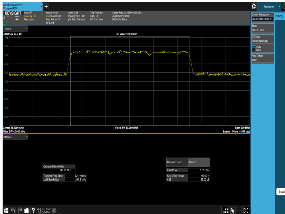
Plot 7-337. Ant M0 OBW (Band n260-50MHz-3CC SISO CP-OFDM – QPSK – Mid Channel)
