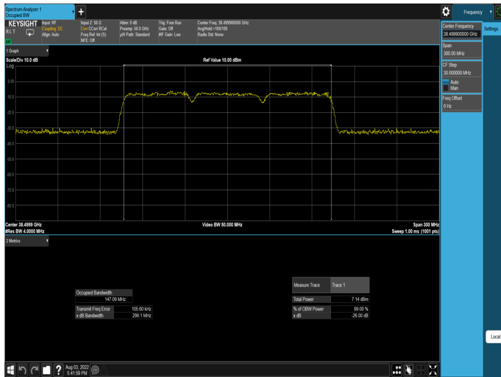
Plot 7-343. Ant M0 OBW (Band n260-50MHz-3CC SISO DFTs-OFDM – 64QAM – Mid Channel)
