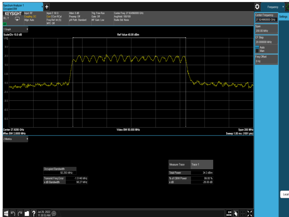
Plot 7-264. Ant M0 OBW (Band n261-100MHz-1CC SISO Dual Pol DFTs-OFDM – QPSK – Mid Channel)
