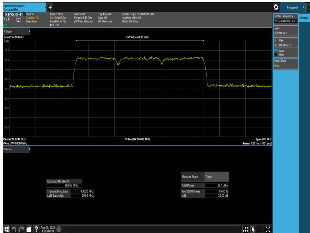
Plot 7-286. Ant M0 OBW (Band n261-100MHz-3CC SISO DFTs-OFDM – 16QAM – Mid Channel)
