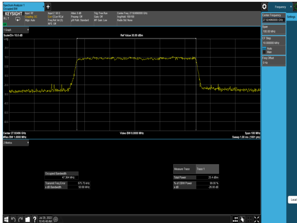
Plot 7-199. Ant M0 OBW (Band n261-50MHz-1CC SISO CP-OFDM – 64QAM – Mid Channel)
