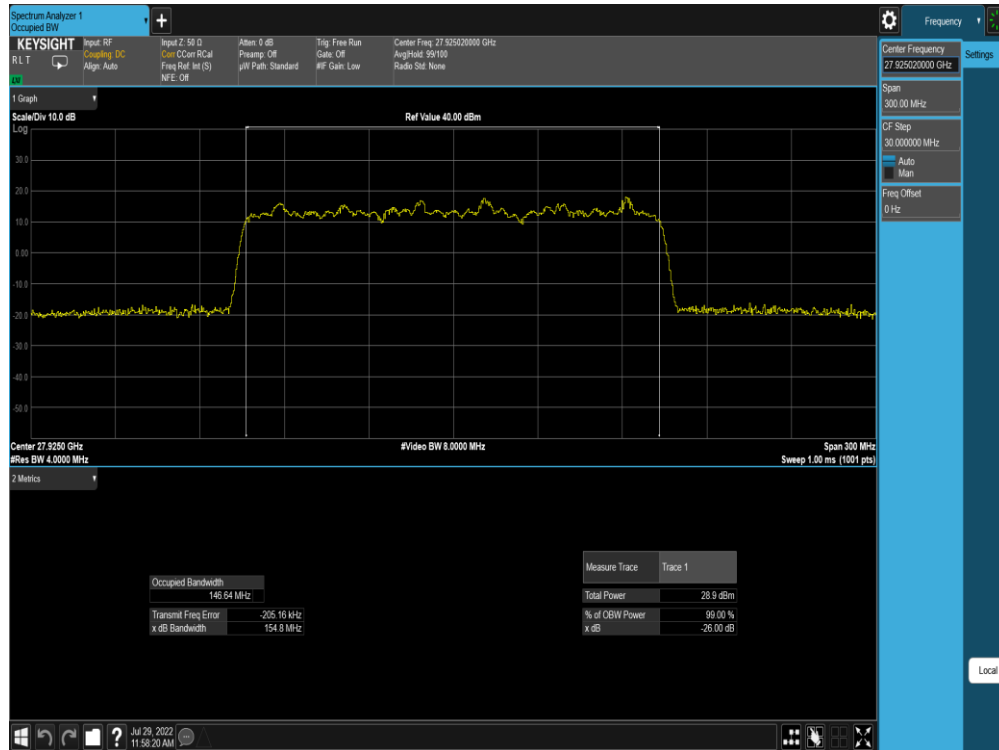
Plot 7-235. Ant M0 OBW (Band n261-50MHz-3CC SISO Dual Pol DFTs-OFDM – \pi/2 BPSK – Mid Channel)
