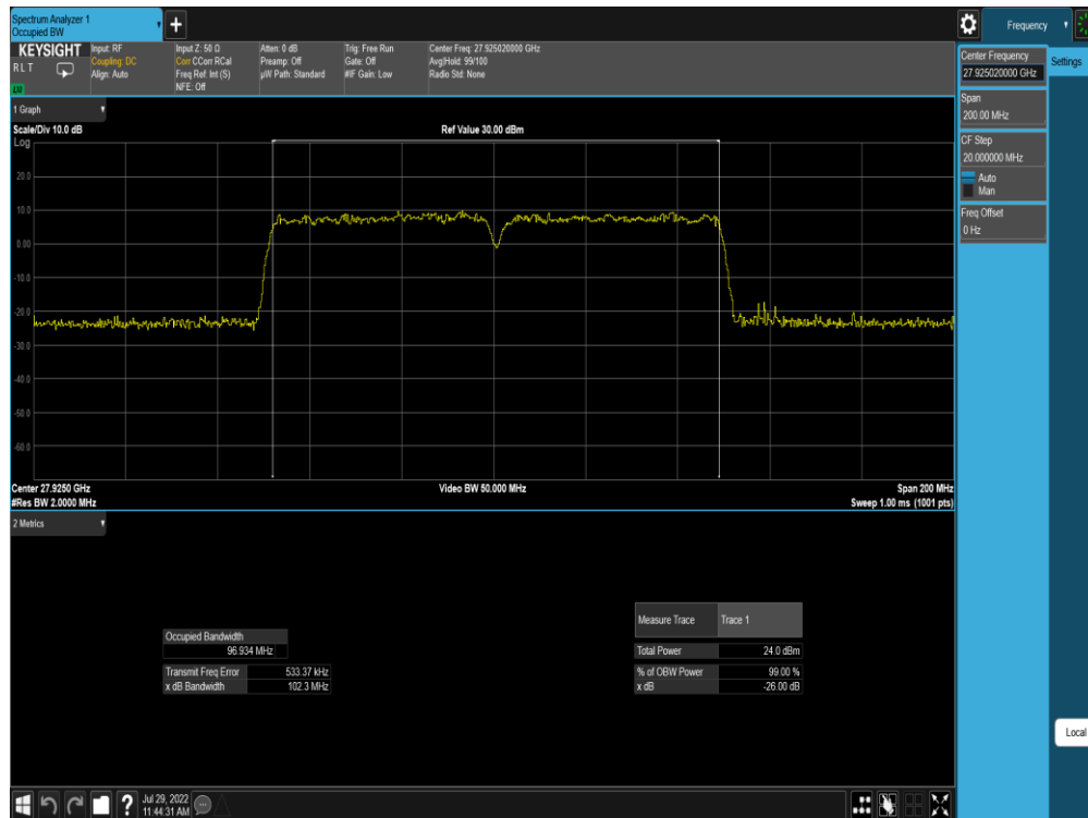
Plot 7-213. Ant M0 OBW (Band n261-50MHz-2CC SISO CP-OFDM – 64QAM – Mid Channel)
