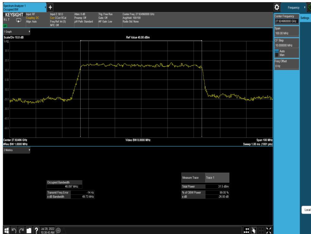
Plot 7-200. Ant M0 OBW (Band n261-50MHz-1CC SISO DFTs-OFDM – \pi/2 BPSK – Mid Channel)
