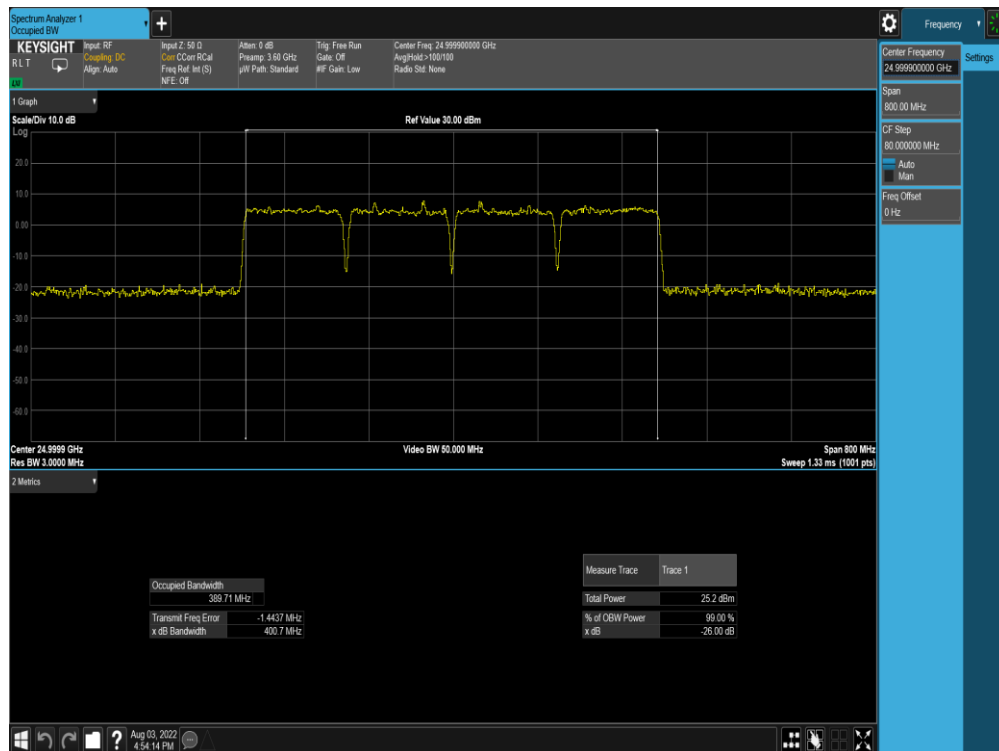
Plot 7-186. Ant M0 OBW (Band n258-R2-100MHz-4CC SISO DFTs-OFDM - \pi/2 BPSK - Mid Channel)
