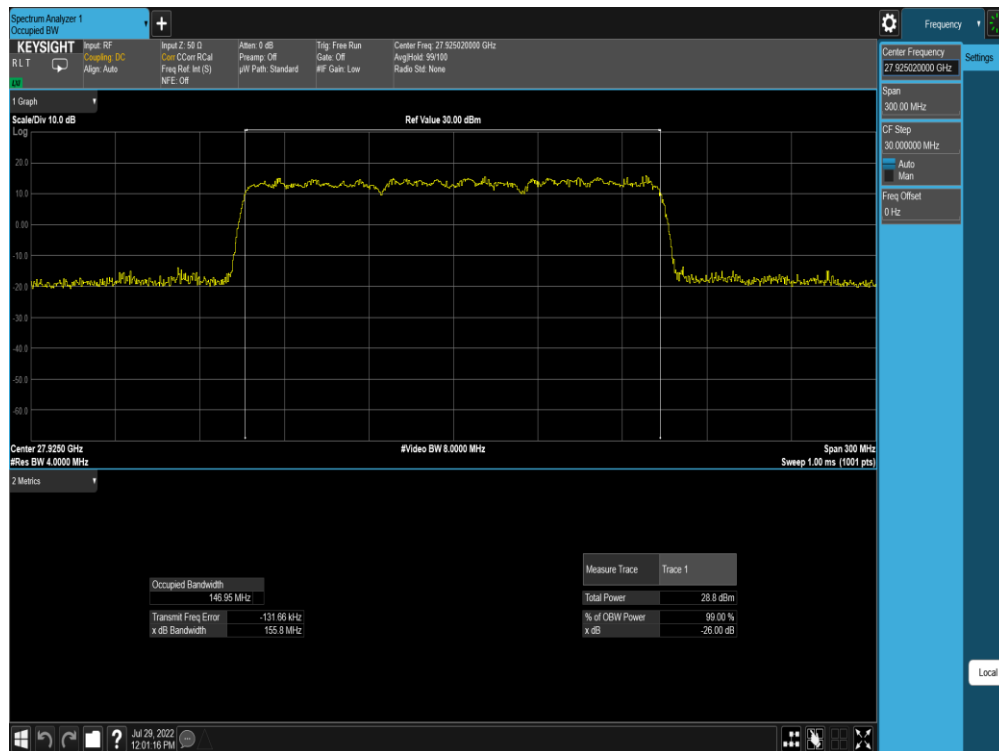
Plot 7-236. Ant M0 OBW (Band n261-50MHz-3CC SISO Dual Pol DFTs-OFDM – QPSK – Mid Channel)
