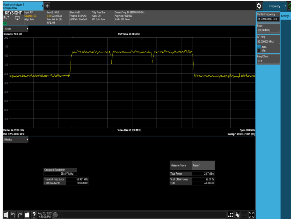
Plot 7-171. Ant M0 OBW (Band n258-R2-100MHz-3CC SISO CP-OFDM – 64QAM – Mid Channel)
