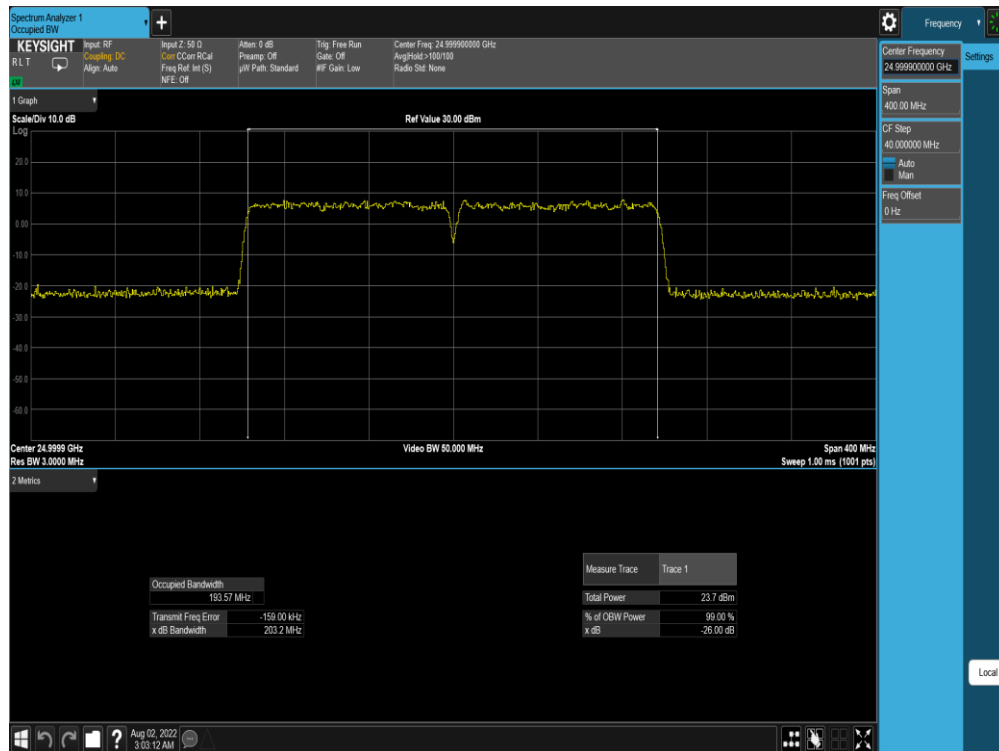
Plot 7-157. Ant M0 OBW (Band n258-R2-100MHz-2CC SISO CP-OFDM – 64QAM – Mid Channel)
