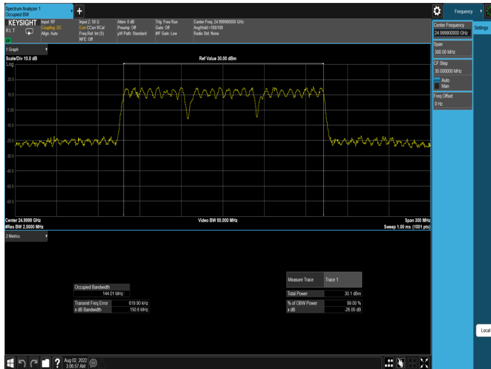
Plot 7-123. Ant M0 OBW (Band n258-R2-50MHz-3CC SISO Dual Pol DFTs-OFDM – \pi/2 BPSK – Mid Channel)
