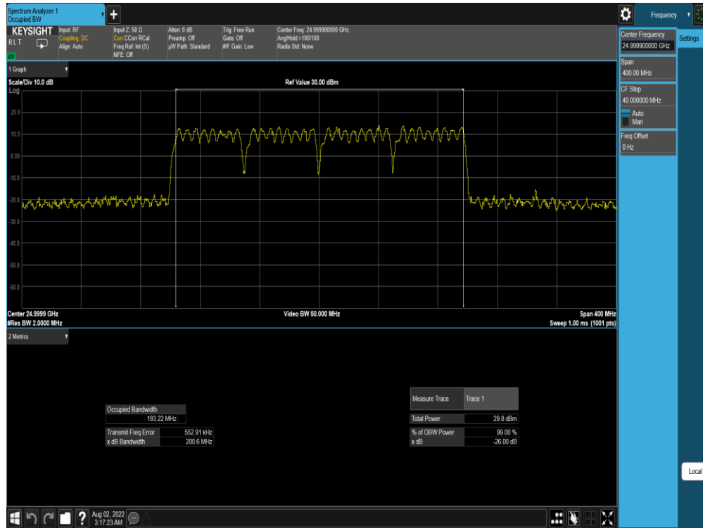
Plot 7-137. Ant M0 OBW (Band n258-R2-50MHz-4CC SISO Dual Pol DFTs-OFDM – \pi/2 BPSK – Mid Channel)
