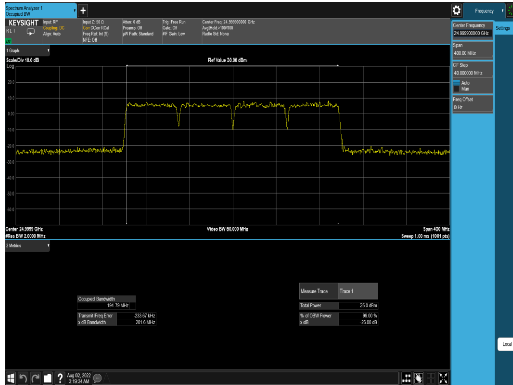
Plot 7-131. Ant M0 OBW (Band n258-R2-50MHz-4CC SISO DFTs-OFDM – QPSK – Mid Channel)
