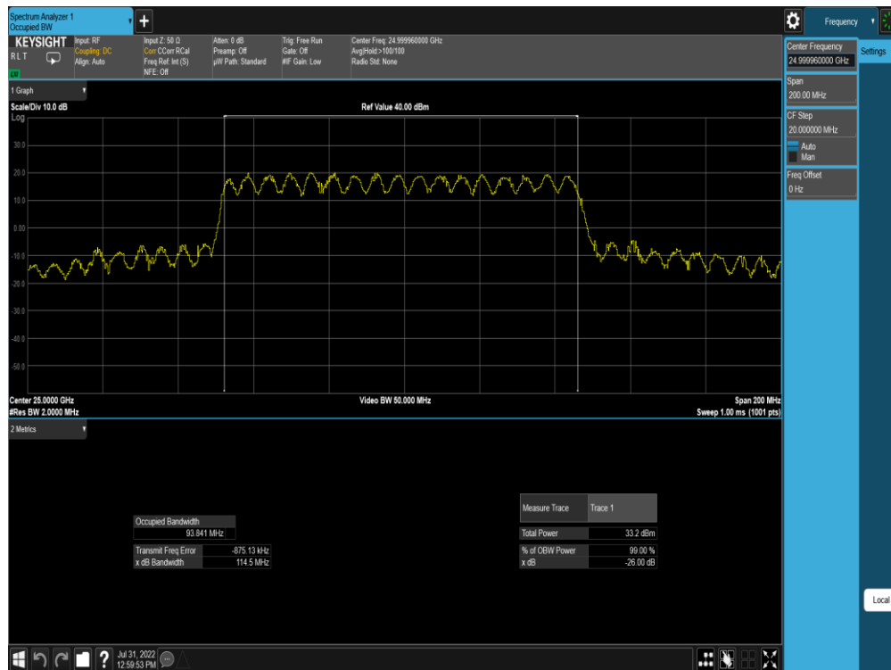
Plot 7-148. Ant M0 OBW (Band n258-R2-100MHz-1CC MIMO CP-OFDM – QPSK – Mid Channel)
