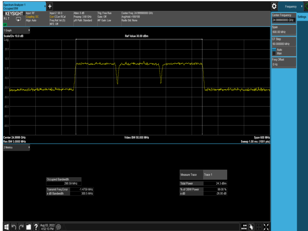
Plot 7-175. Ant M0 OBW (Band n258-R2-100MHz-3CC SISO DFTs-OFDM – 64QAM – Mid Channel)
