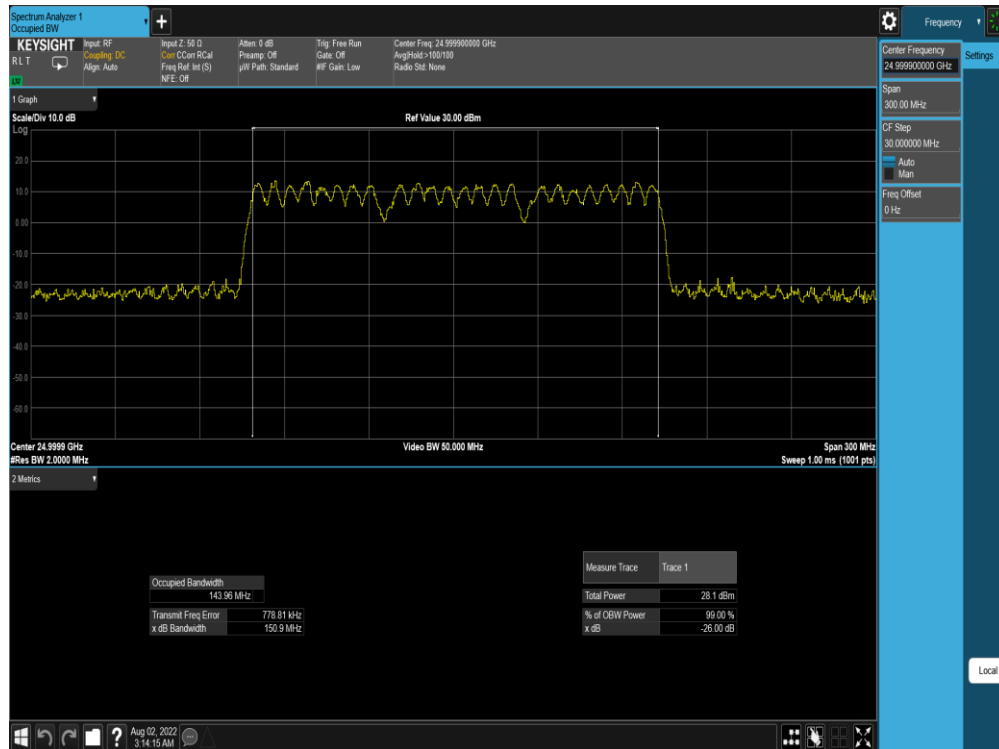
Plot 7-122. Ant M0 OBW (Band n258-R2-50MHz-3CC MIMO CP-OFDM - 64QAM - Mid Channel)
