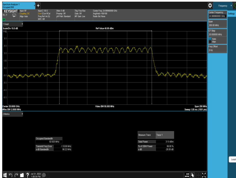
Plot 7-154. Ant M0 OBW (Band n258-R2-100MHz-1CC SISO Dual Pol DFTs-OFDM – 64QAM – Mid Channel)
