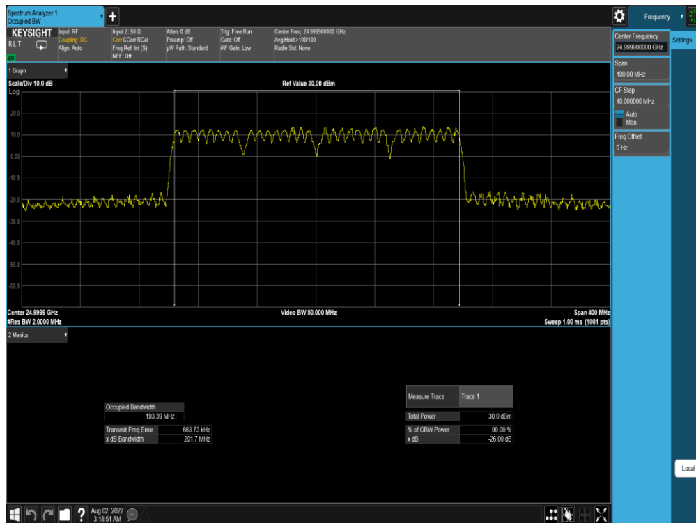
Plot 7-134. Ant M0 OBW (Band n258-R2-50MHz-4CC MIMO CP-OFDM – QPSK – Mid Channel)
