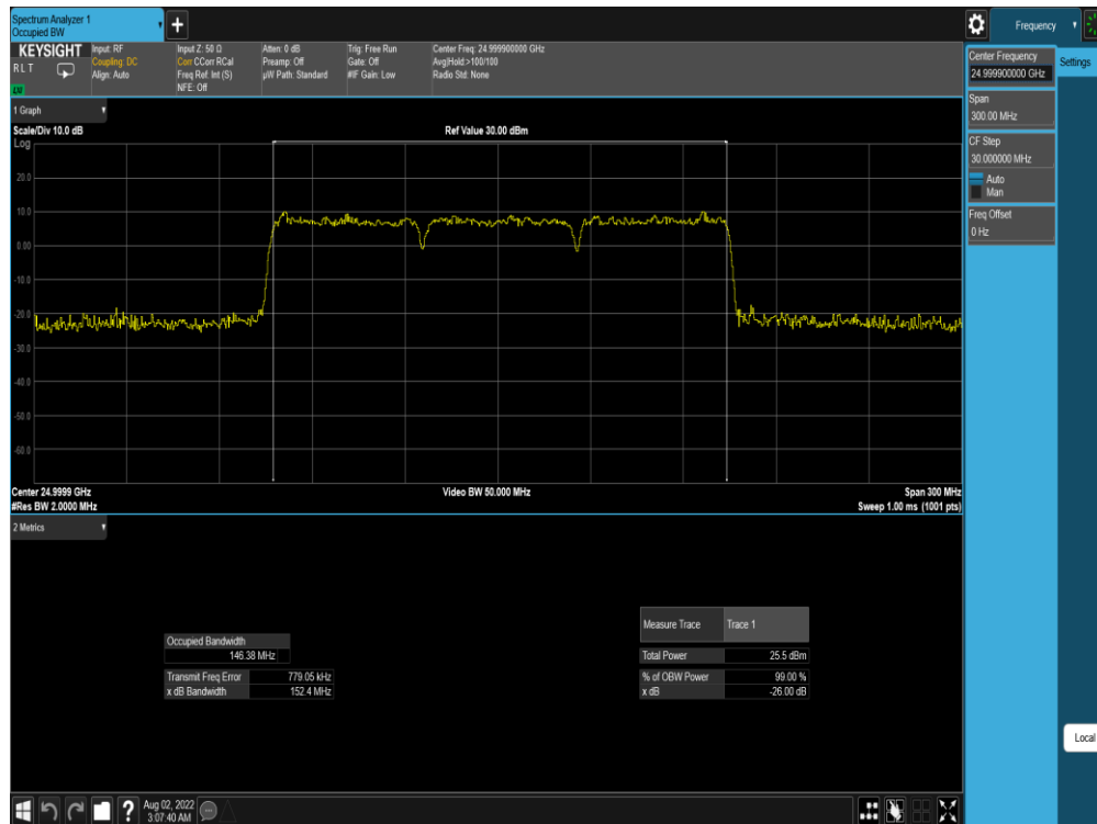
Plot 7-113. Ant M0 OBW (Band n258-R2-50MHz-3CC SISO CP-OFDM – QPSK – Mid Channel)
