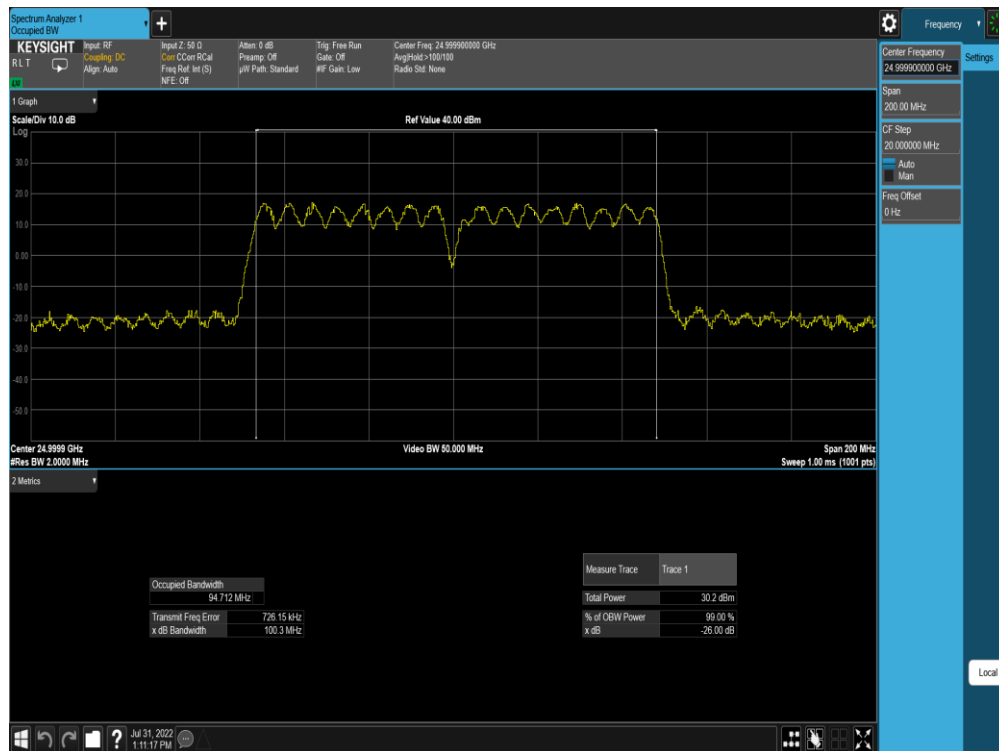
Plot 7-110. Ant M0 OBW (Band n258-R2-50MHz-2CC SISO Dual Pol DFTs-OFDM – QPSK – Mid Channel)
