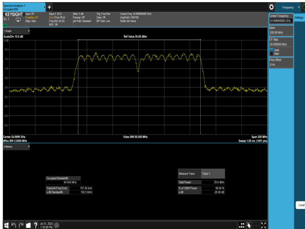
Plot 7-112. Ant M0 OBW (Band n258-R2-50MHz-2CC SISO Dual Pol DFTs-OFDM – 64QAM – Mid Channel)
