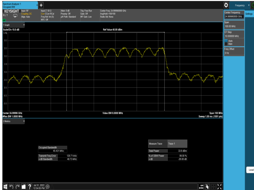
Plot 7-97. Ant M0 OBW (Band n258-R2-50MHz-1CC SISO Dual Pol DFTs-OFDM – 16QAM – Mid Channel)
