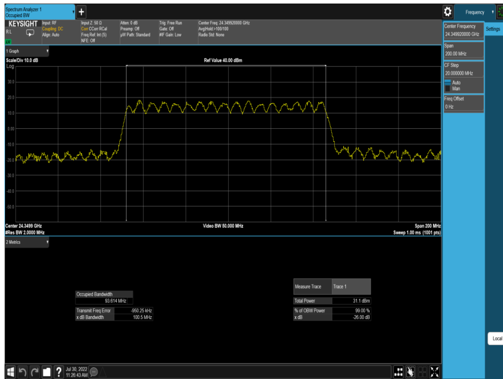
Plot 7-65. Ant M0 OBW (Band n258-R1-100MHz-1CC MIMO CP-OFDM – 16QAM – Mid Channel)
