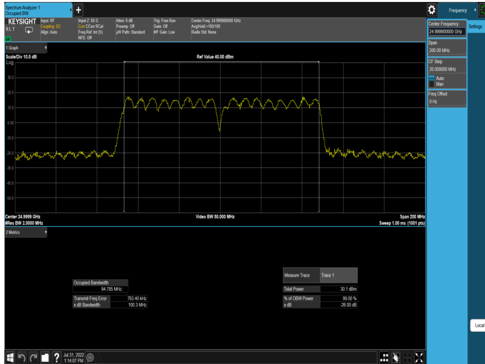
Plot 7-111. Ant M0 OBW (Band n258-R2-50MHz-2CC SISO Dual Pol DFTs-OFDM – 16QAM – Mid Channel)
