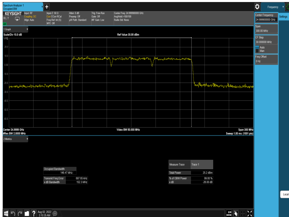
Plot 7-114. Ant M0 OBW (Band n258-R2-50MHz-3CC SISO CP-OFDM – 16QAM – Mid Channel)
