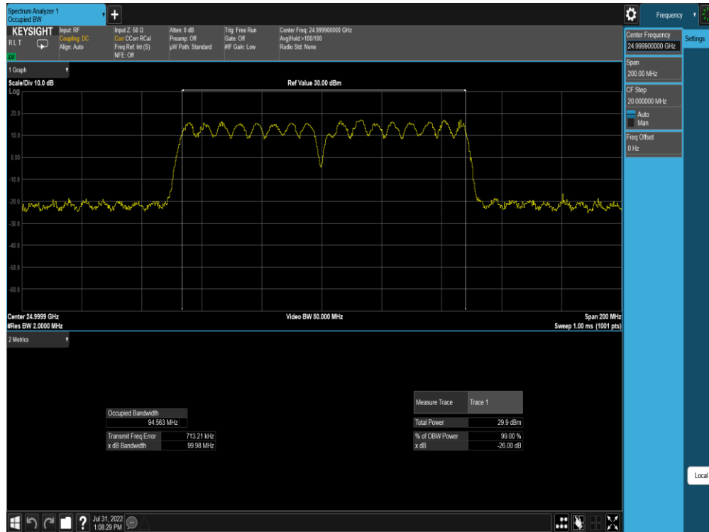
Plot 7-109. Ant M0 OBW (Band n258-R2-50MHz-2CC SISO Dual Pol DFTs-OFDM – \pi/2 BPSK – Mid Channel)
