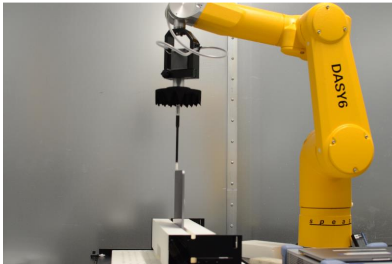
Test Setup Photo 8 – Power Density Measurement Setup (Figure 7-2)
