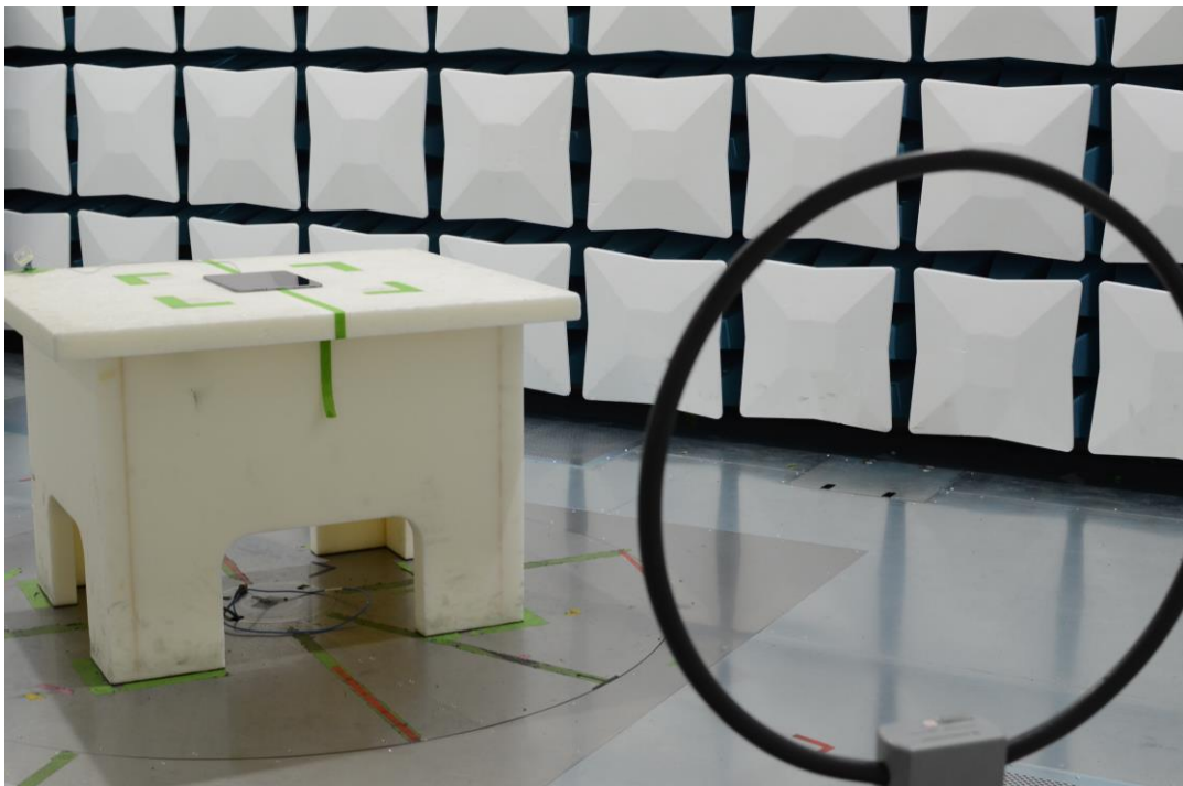
Figure 23: 9kHz-30MHz Test Setup (Front View)
