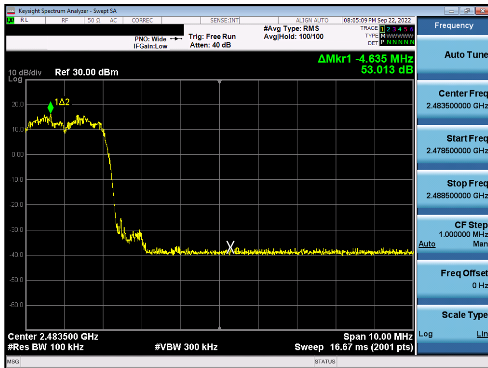
Plot 7-20. Band Edge Plot Antenna 4a (Bluetooth with Hopping Enabled, 8DPSK, ePA, 2.4GHz)
