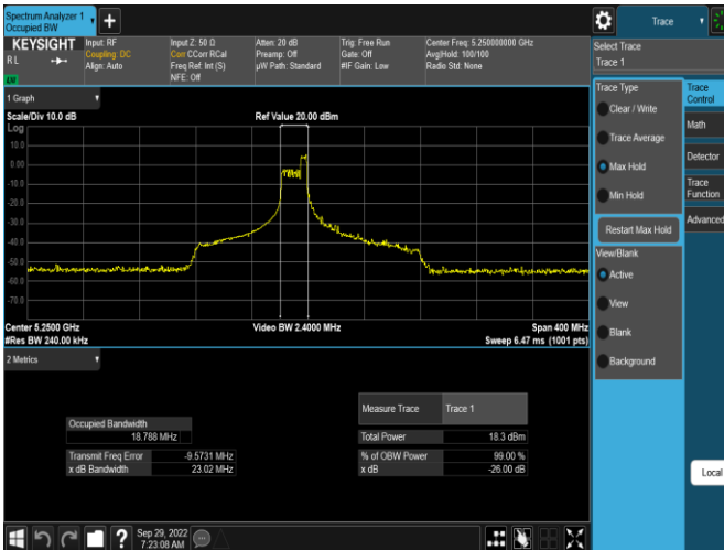
Plot 7-14. 26dB BW & 99% OBW Antenna WF5b (160MHz BW 11ax Index 52 - RU52 - Ch.50(L))
