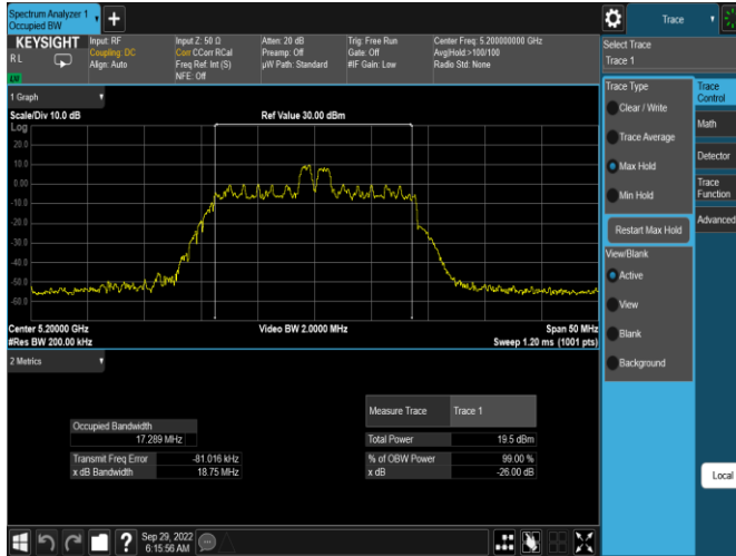
Plot 7-2. 26dB BW & 99% OBW Antenna WF5b (20MHz BW 11ax Index 4 – RU26 – Ch.40)
