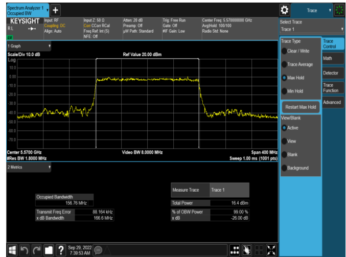
Plot 7-44. 26dB BW & 99% OBW Antenna WF5b (160MHz BW 11ax – RU996x2 – Ch.114)
