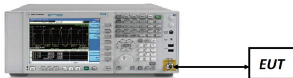
Figure 7-1. Test Instrument & Measurement Setup
