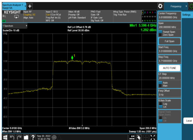
Plot 7-467. PSD CDD Antenna 5b (80MHz BW 802.11ax(SU) – Ch. 122, MCS4 (FCC))
