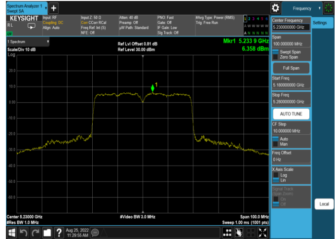
Plot 7-272. ISED PSD Antenna 5b (40MHz BW 11ax(SU) – Ch.46, MCS11)
