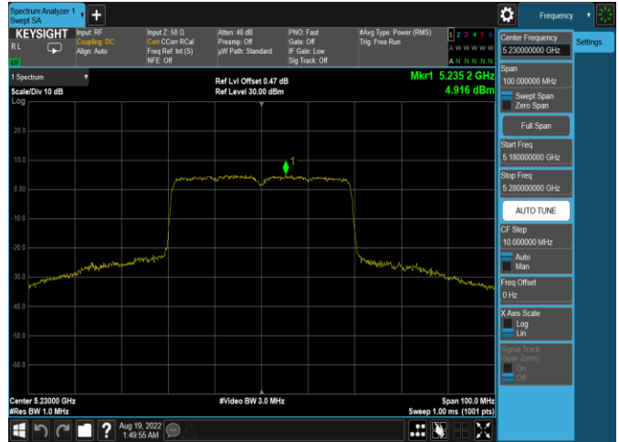
Plot 7-264. ISED PSD Antenna 5b (40MHz BW 11ax(SU) – Ch.46, MCS4)
