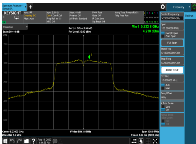
Plot 7-263. ISED PSD Antenna 5b (40MHz BW 11n – Ch.46, MCS4)
