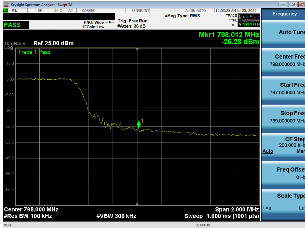
Plot 7-94. Upper Band Edge Plot (LTE Band 14, 10MHz QPSK - RB Size 50)
