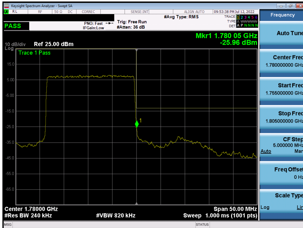
Plot 7-311. Upper Band Edge Plot (NR Band n66 – 20.0MHz DFT-s-OFDM \pi/2 BPSK - Full RB)
