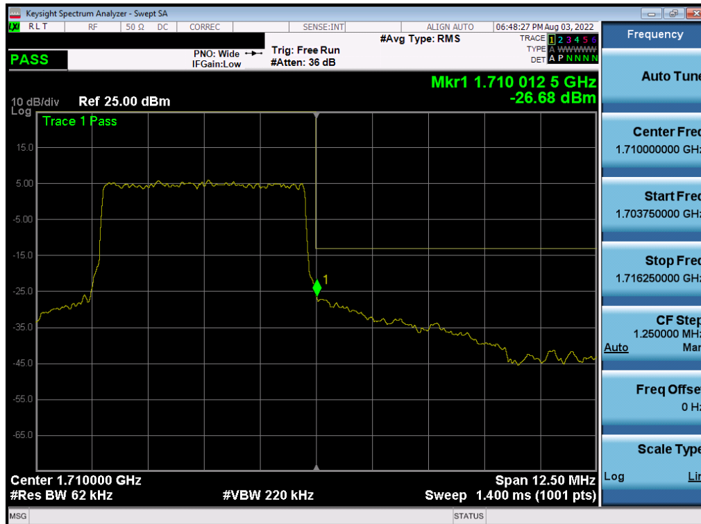
Plot 7-323. Upper Band Edge Plot (NR Band n70 – 5.0MHz DFT-s-OFDM QPSK - Full RB)
