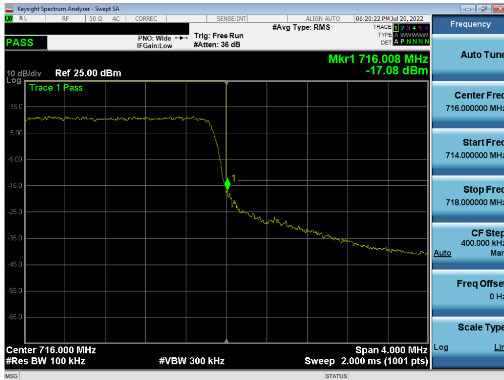
Plot 7-280. Upper Band Edge Plot (LTE Band 12 - 3MHz QPSK – Full RB)
