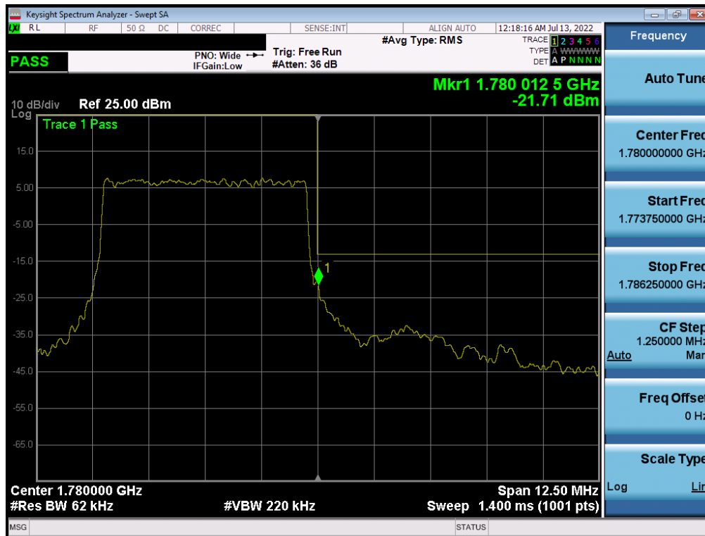
Plot 7-299. Upper Band Edge Plot (NR Band n66 – 5.0MHz DFT-s-OFDM \pi/2 BPSK - Full RB)
