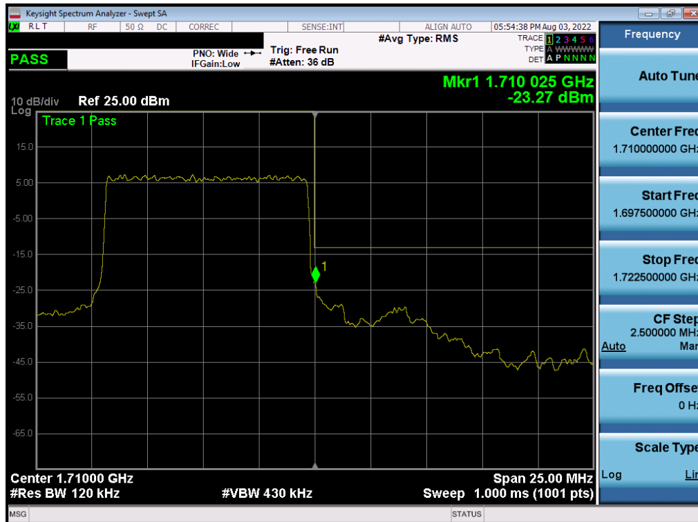
Plot 7-327. Upper Band Edge Plot (NR Band n70 – 10.0MHz DFT-s-OFDM \pi/2 BPSK - Full RB)
