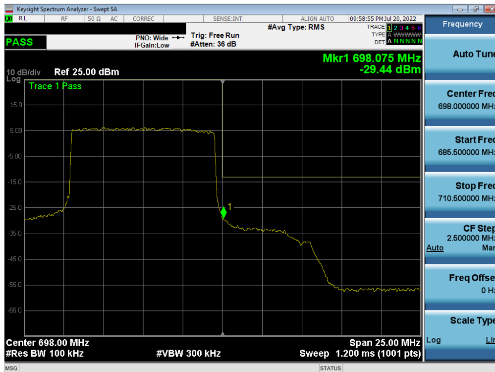
Plot 7-272. Upper Band Edge Plot (LTE Band 71 - 10MHz QPSK - Full RB)
