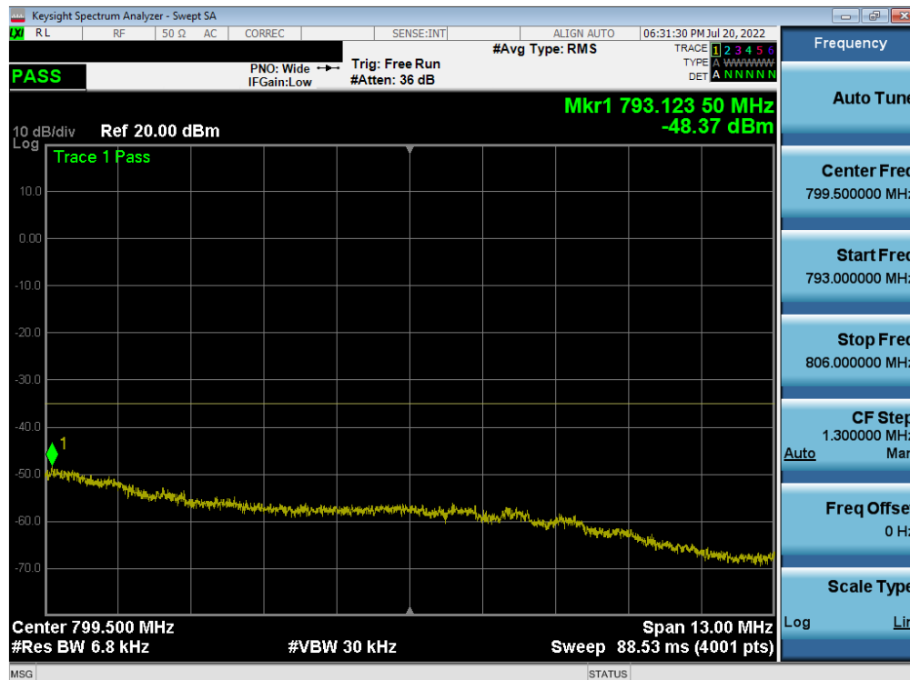
Plot 7-296. Upper Emission Mask Plot (LTE Band 13 - 10MHz QPSK – Full RB)
