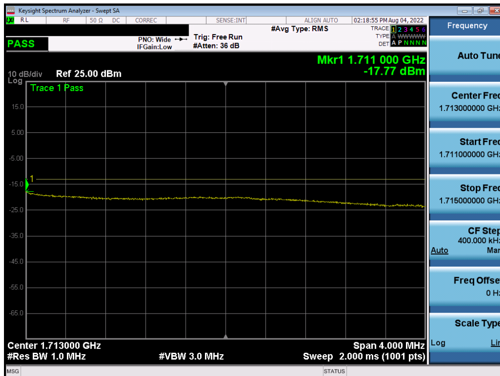
Plot 7-332. Upper Extended Band Edge Plot (NR Band n70 – 15.0MHz DFT-s-OFDM QPSK - Full RB)
