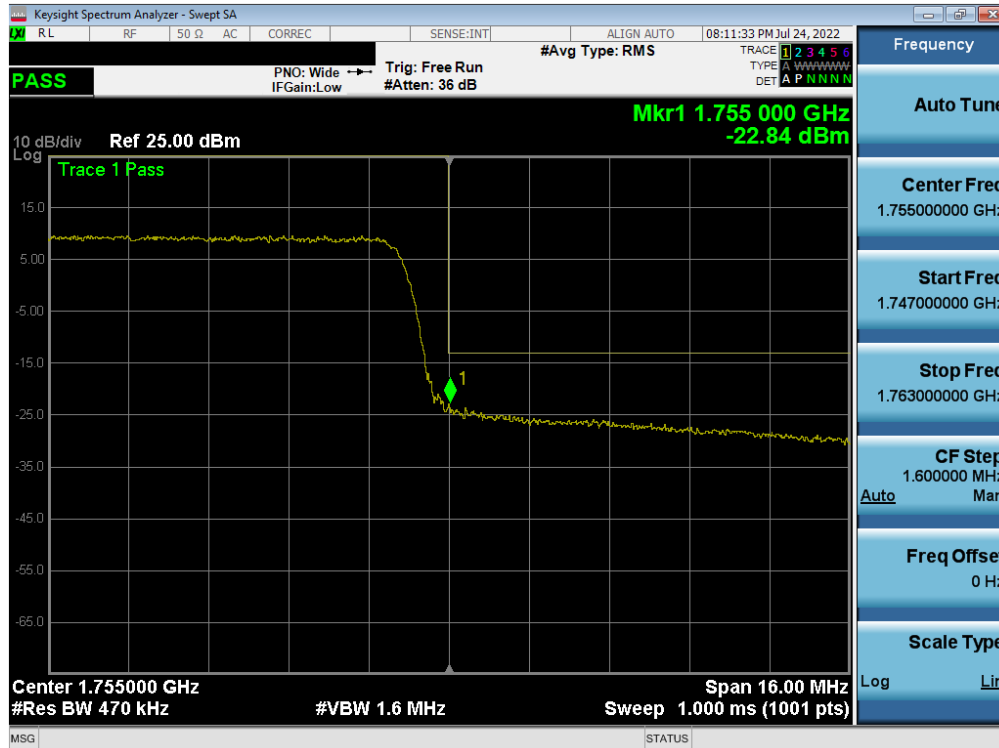
Plot 7-267. Upper Band Edge Plot (LTE Band 4 - 20MHz QPSK – Full RB)
