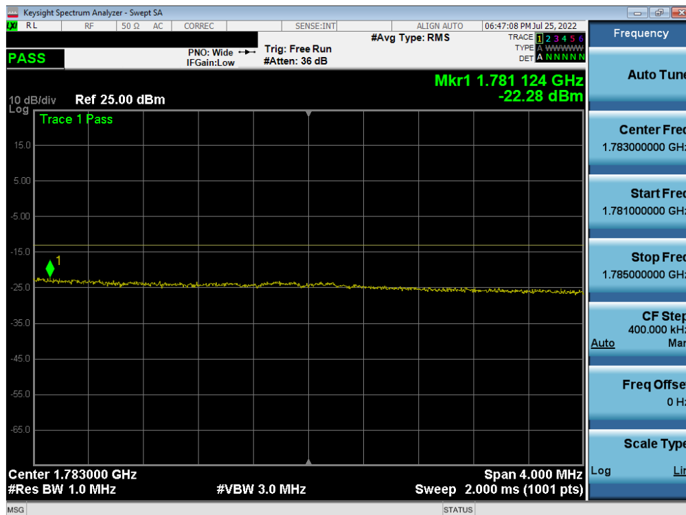
Plot 7-240. Upper Extended Band Edge Plot (LTE Band 66 - 15MHz QPSK - Full RB)
