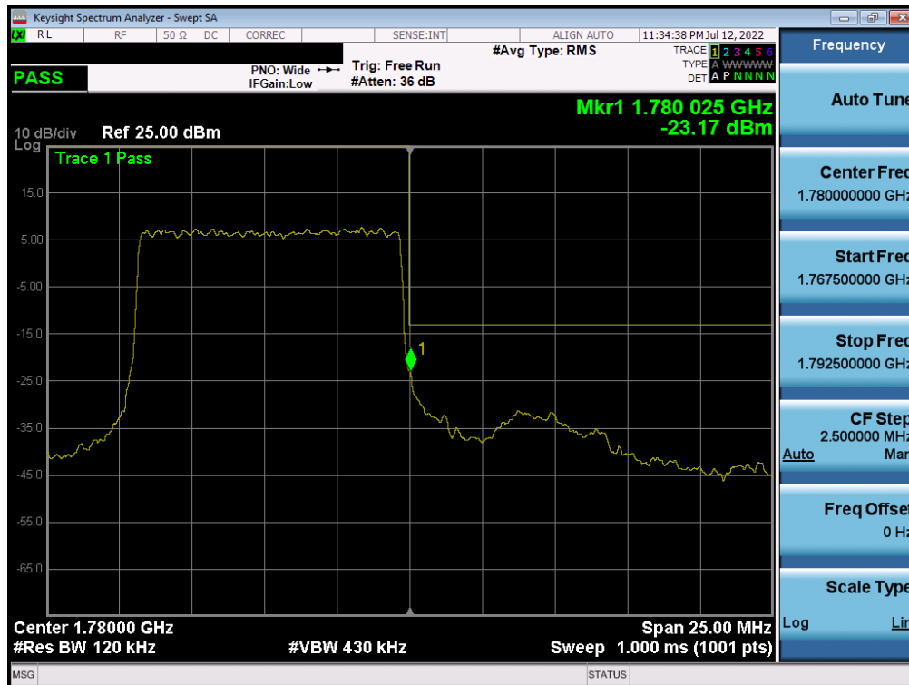
Plot 7-303. Upper Band Edge Plot (NR Band n66 – 10.0MHz DFT-s-OFDM \pi/2 BPSK - Full RB)
