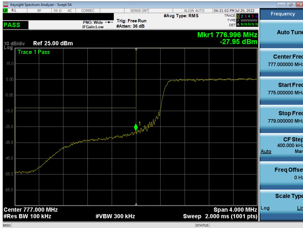
Plot 7-293. Lower Band Edge Plot (LTE Band 13 - 10MHz QPSK – Full RB)
