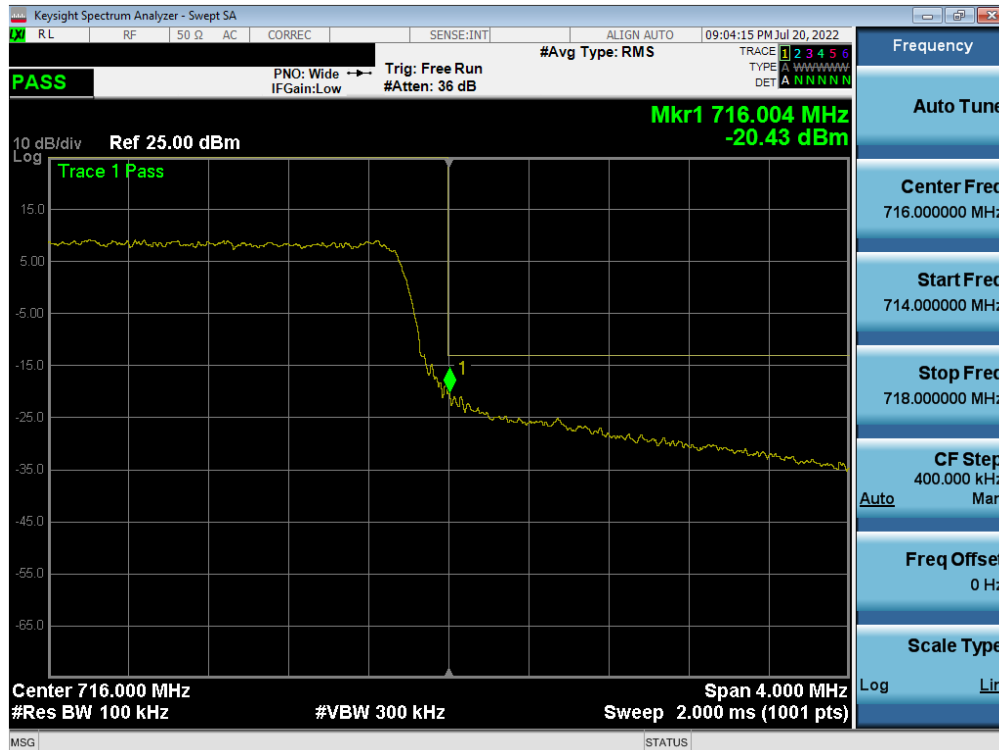
Plot 7-286. Upper Band Edge Plot (LTE Band 17 - 5MHz QPSK – Full RB)
