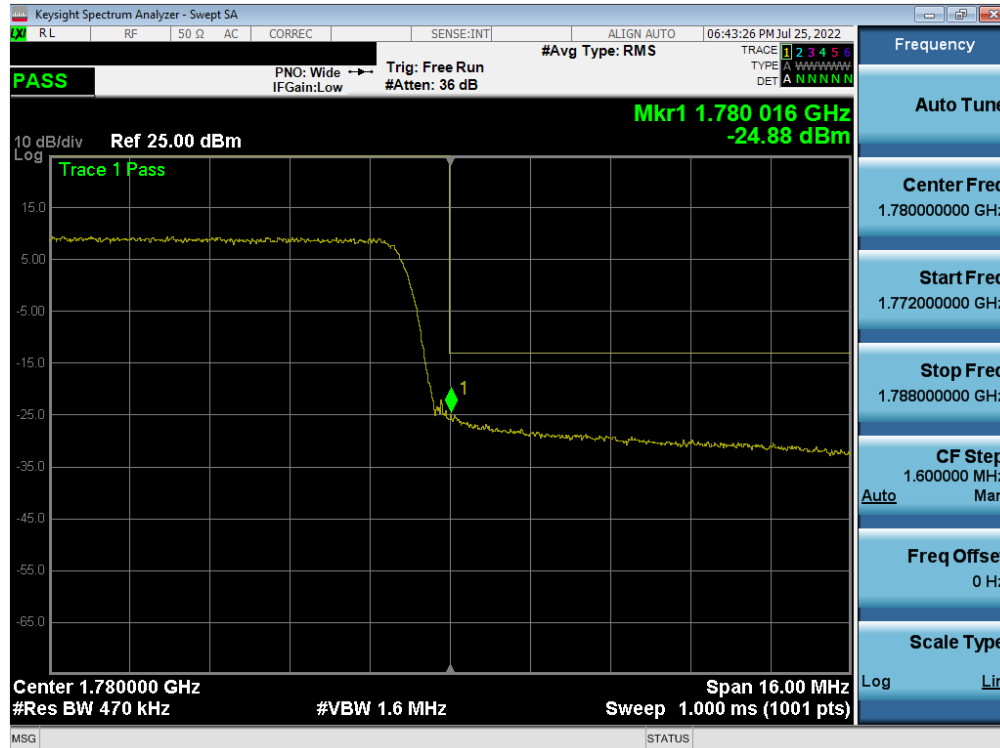
Plot 7-243. Upper Band Edge Plot (LTE Band 66 - 20MHz QPSK - Full RB)
