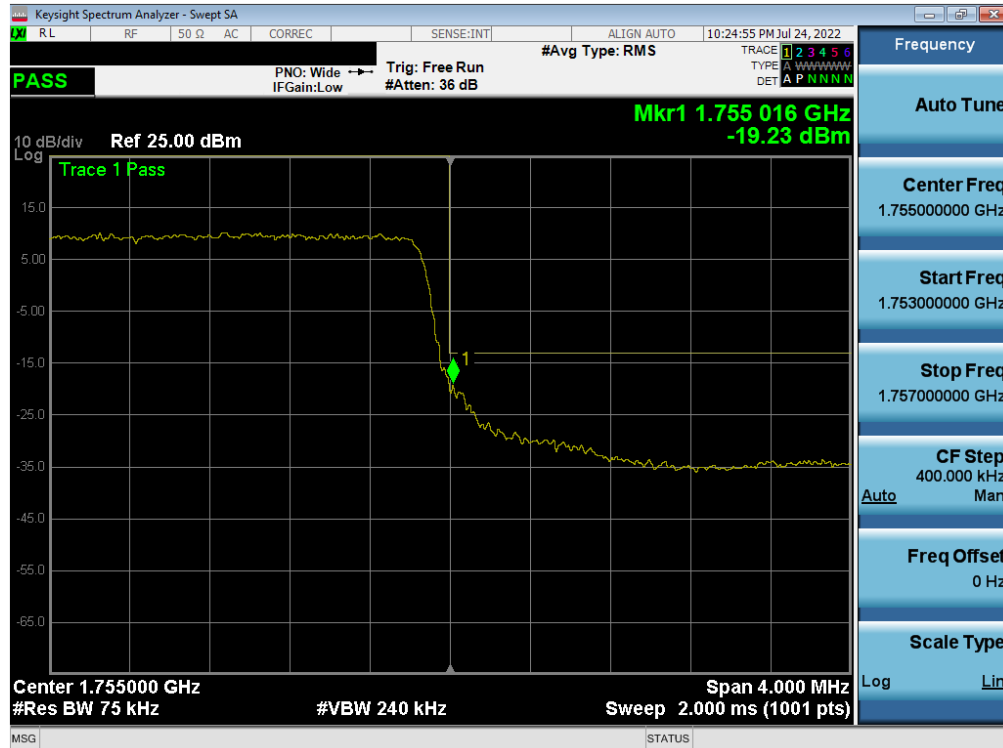
Plot 7-251. Upper Band Edge Plot (LTE Band 4 - 3MHz QPSK – Full RB)
