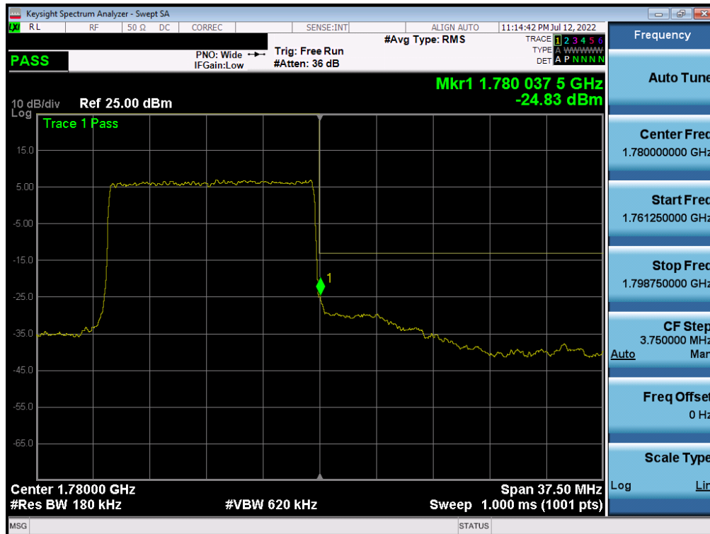
Plot 7-307. Upper Band Edge Plot (NR Band n66 – 15.0MHz DFT-s-OFDM \pi/2 BPSK - Full RB)
