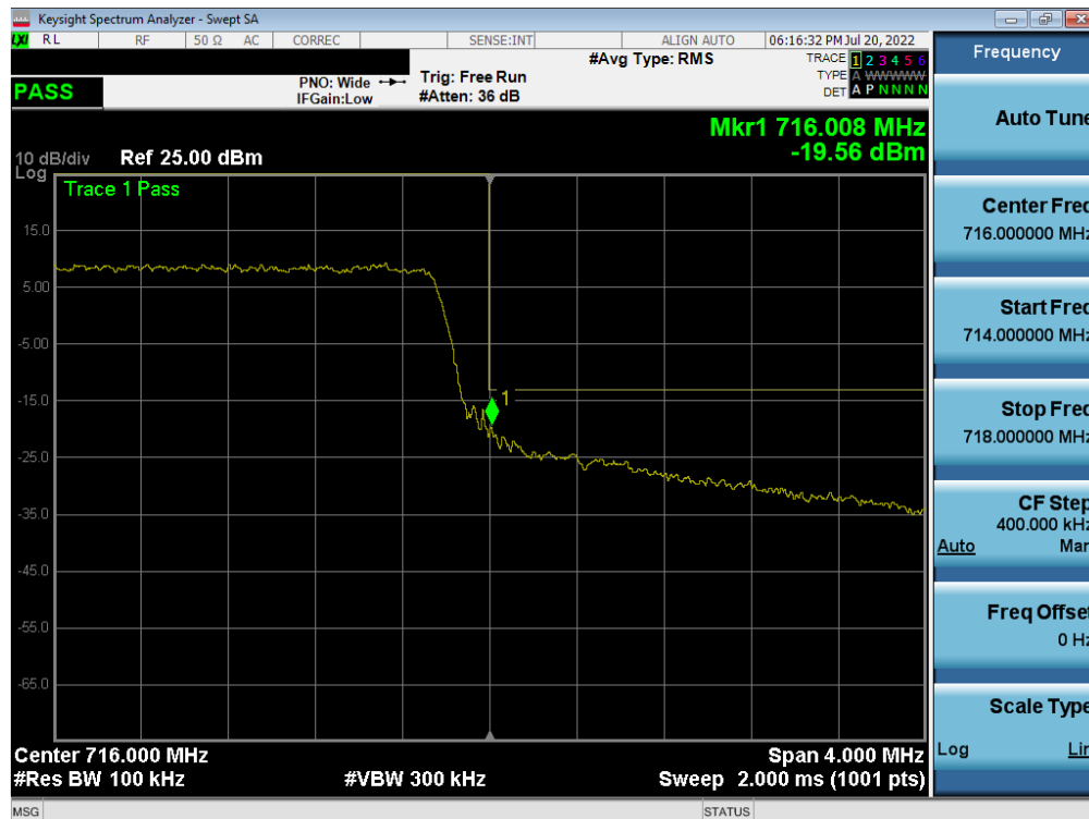
Plot 7-282. Upper Band Edge Plot (LTE Band 12 - 5MHz QPSK - Full RB)
