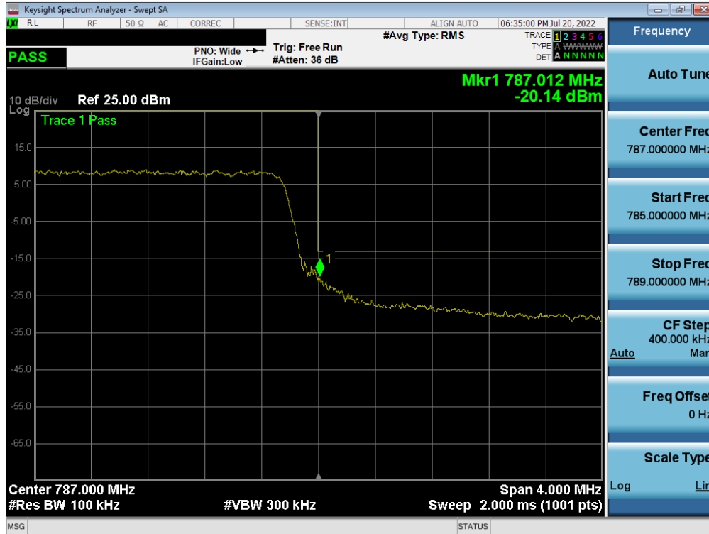
Plot 7-291. Upper Band Edge Plot (LTE Band 13 - 5MHz QPSK – Full RB)
