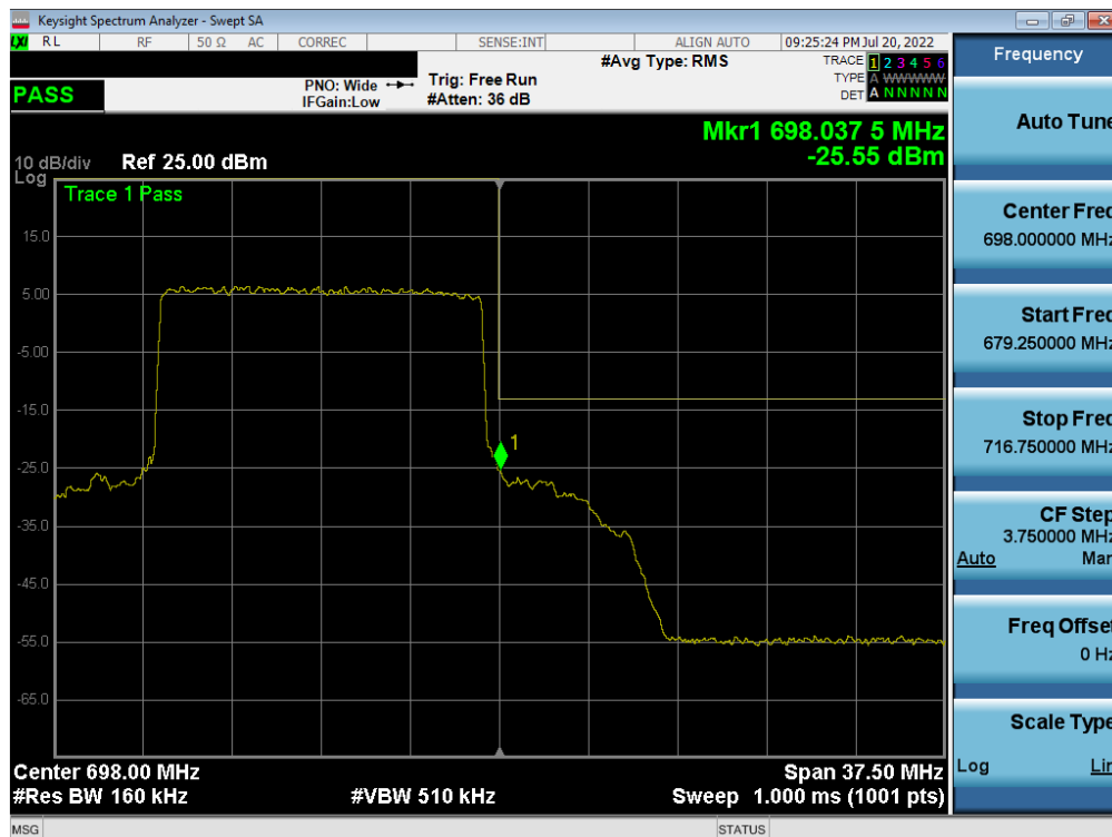
Plot 7-274. Upper Band Edge Plot (LTE Band 71 - 15MHz QPSK – Full RB)
