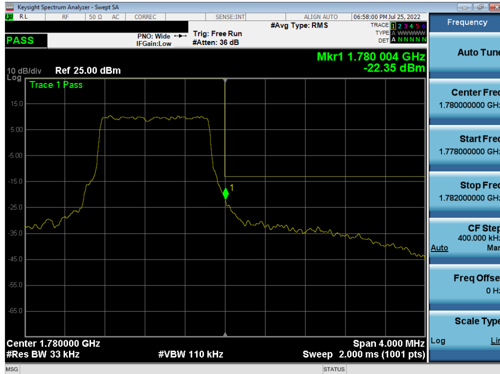
Plot 7-223. Upper Band Edge Plot (LTE Band 66 – 1.4MHz QPSK – Full RB)
