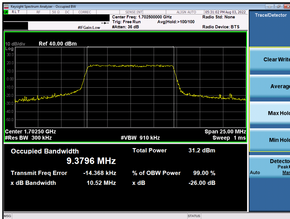
Plot 7-102. Occupied Bandwidth Plot (NR Band n70 - 10.0MHz CP-OFDM 16QAM - Full RB)
