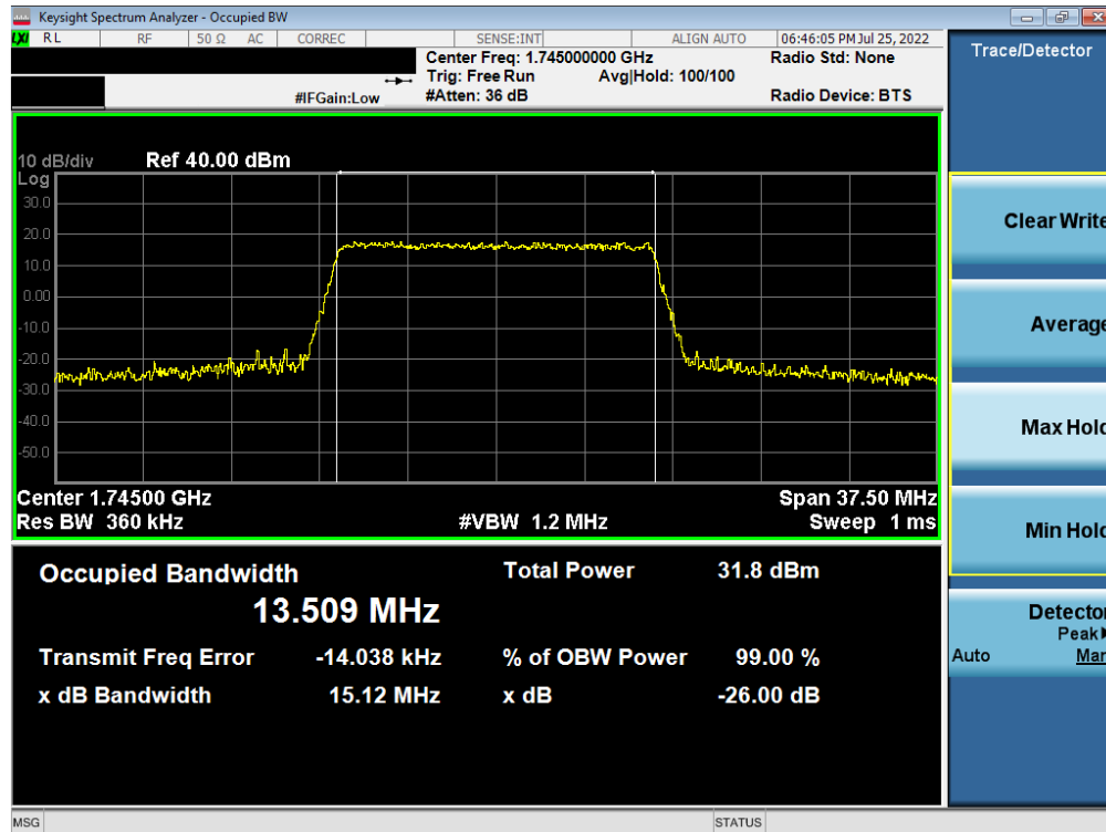
Plot 7-19. Occupied Bandwidth Plot (LTE Band 66/4 - 15MHz 64-QAM - Full RB)
