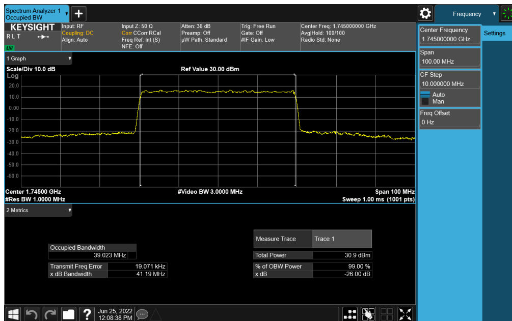
Plot 7-94. Occupied Bandwidth Plot (NR Band n66 - 40.0MHz DFT-s-OFDM 256QAM - Full RB)
