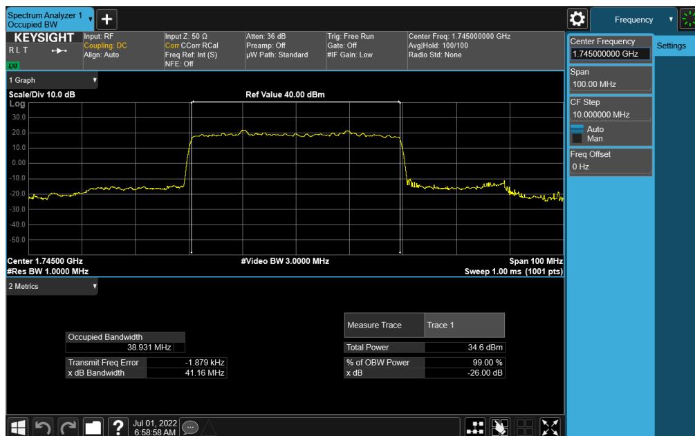
Plot 7-90. Occupied Bandwidth Plot (NR Band n66 - 40.0MHz DFT-s-OFDM \pi/2 BPSK - Full RB)
