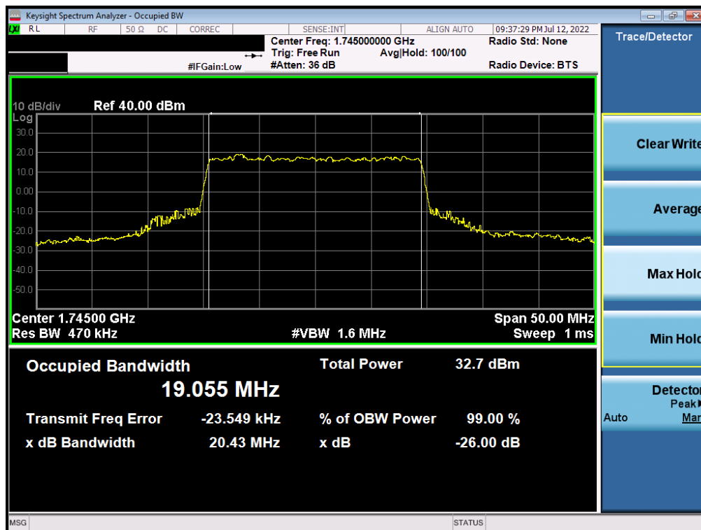
Plot 7-82. Occupied Bandwidth Plot (NR Band n66 - 20.0MHz CP-OFDM 16QAM - Full RB)
