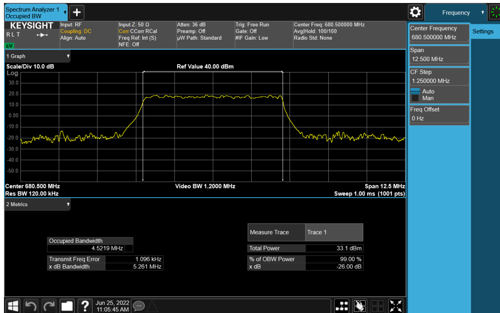
Plot 7-111. Occupied Bandwidth Plot (NR Band n71 - 5MHz CP-OFDM QPSK - Full RB)
