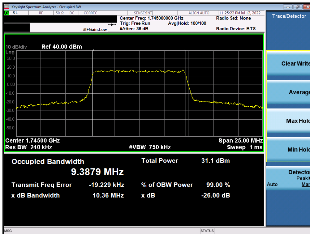
Plot 7-72. Occupied Bandwidth Plot (NR Band n66 - 10.0MHz CP-OFDM 16QAM - Full RB)
