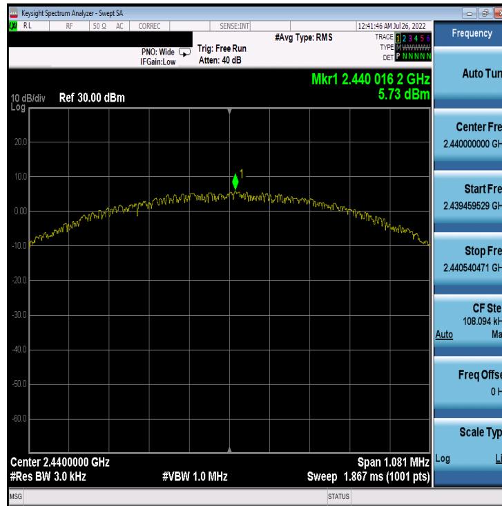
Plot 7-17. Power Spectral Density Plot Antenna 4a (Bluetooth (LE), 1Mbps, iPA – Ch. 19)
