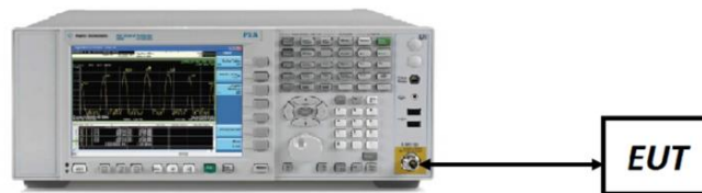
Figure 7-5. Test Instrument & Measurement Setup
