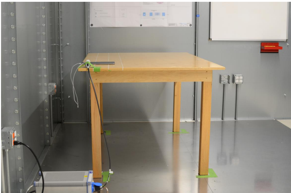
Figure 2: AC Line Conducted Emissions (Side View)
