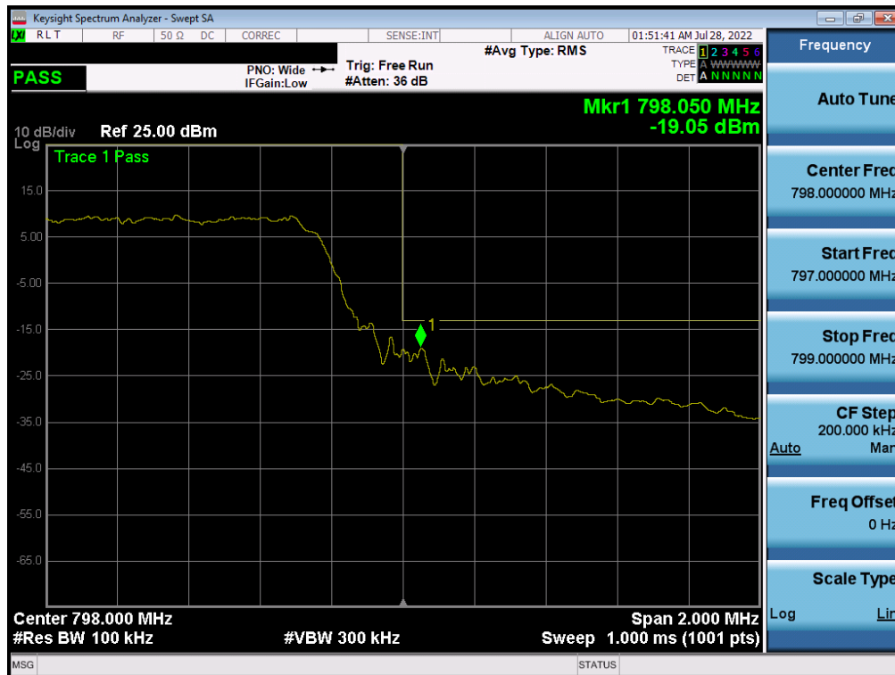
Plot 7-98. Upper Band Edge Plot (NR Band n14, 5MHz DFT-s-OFDM \pi/2 BPSK - RB Size 25)
