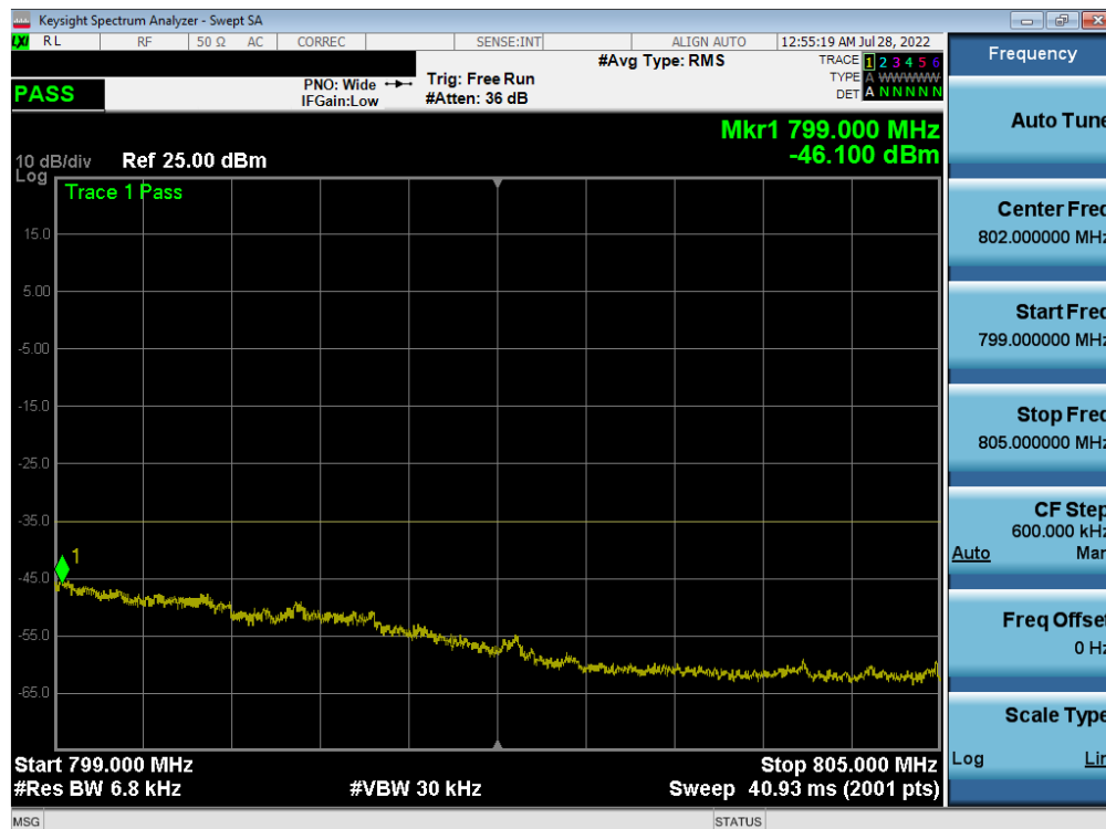
Plot 7-91. Upper Emission Mask Plot (LTE Band 14, 5MHz QPSK - RB Size 25)
