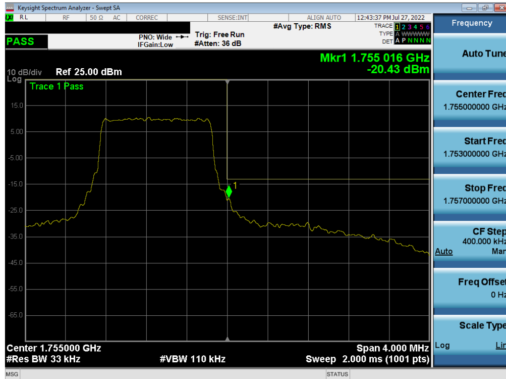
Plot 7-247. Upper Band Edge Plot (LTE Band 4 – 1.4MHz QPSK – Full RB)
