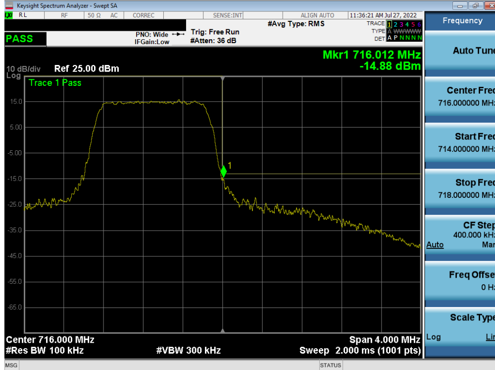
Plot 7-278. Upper Band Edge Plot (LTE Band 12 – 1.4MHz QPSK – Full RB)
