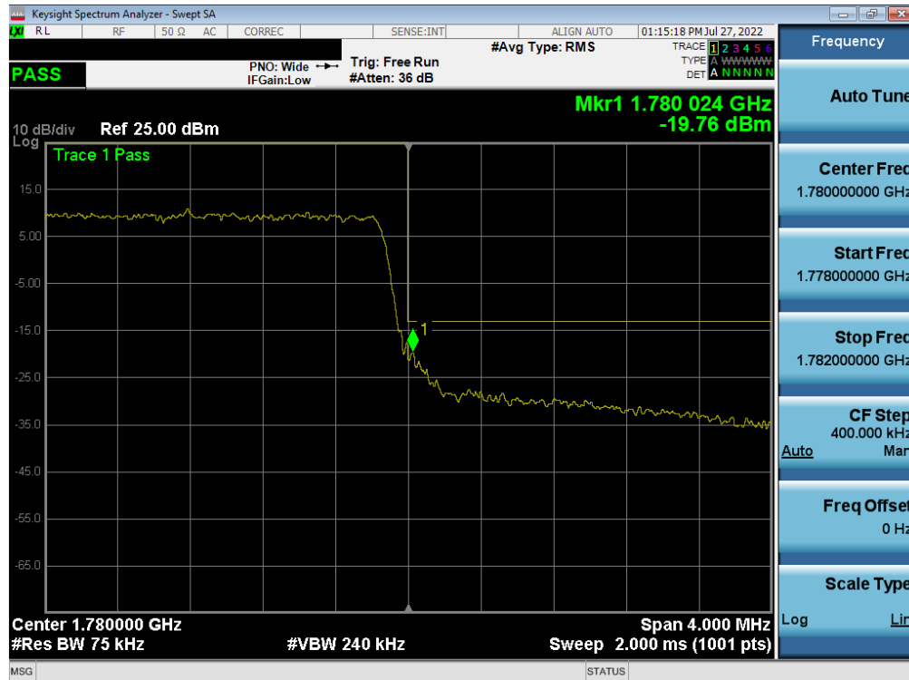
Plot 7-227. Upper Band Edge Plot (LTE Band 66 - 3MHz QPSK – Full RB)
