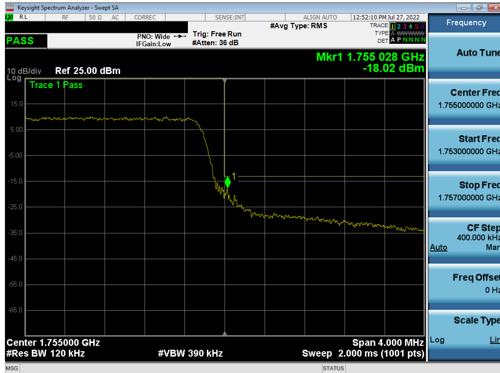
Plot 7-255. Upper Band Edge Plot (LTE Band 4 - 5MHz QPSK – Full RB)
