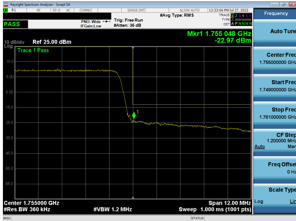
Plot 7-263. Upper Band Edge Plot (LTE Band 4 - 15MHz QPSK – Full RB)
