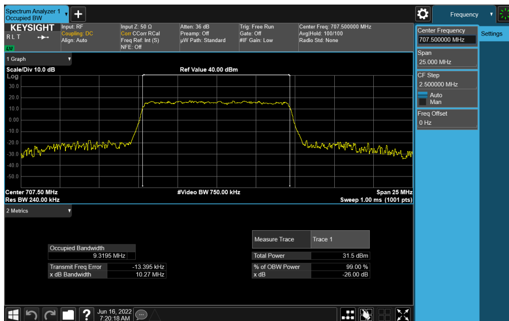
Plot 7-135. Occupied Bandwidth Plot (NR Band n12 - 10MHz DFT-s-OFDM \pi/2 BPSK - Full RB)
