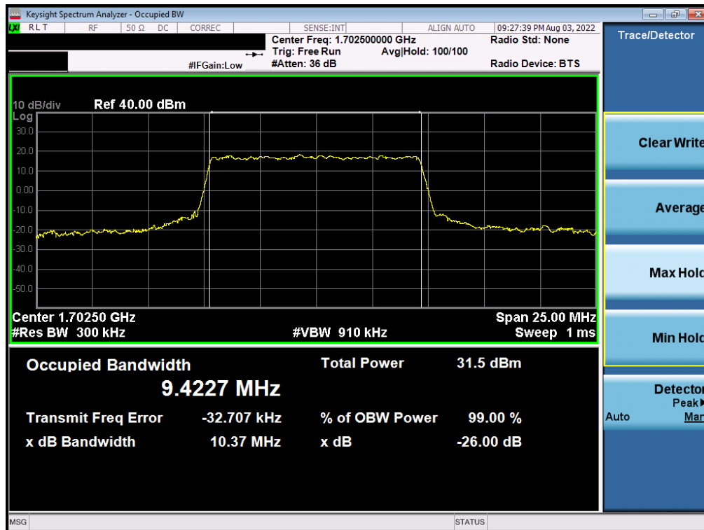
Plot 7-103. Occupied Bandwidth Plot (NR Band n70 - 10.0MHz CP-OFDM 64QAM - Full RB)
