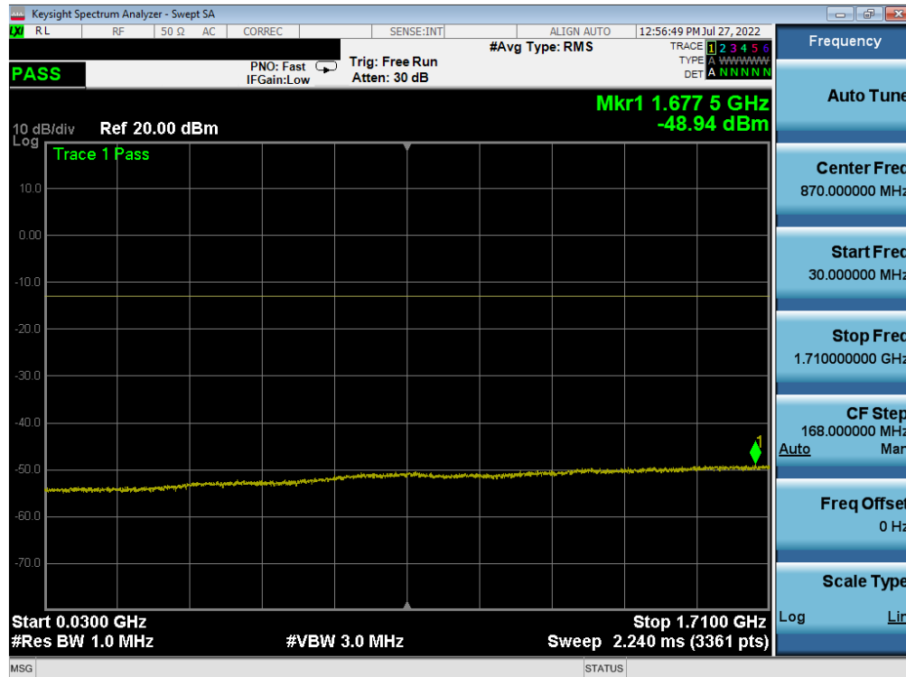
Plot 7-152. Conducted Spurious Plot (LTE Band 66/4 - 20MHz QPSK - RB Size 1, RB Offset 0 - High Channel)
