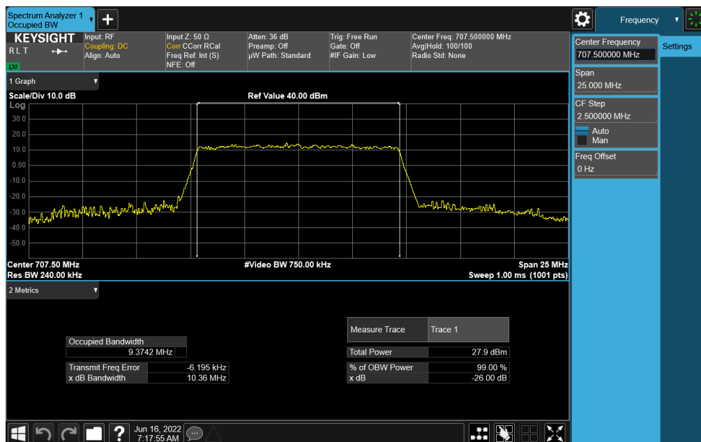
Plot 7-139. Occupied Bandwidth Plot (NR Band n12 - 10MHz CP-OFDM 256-QAM - Full RB)
