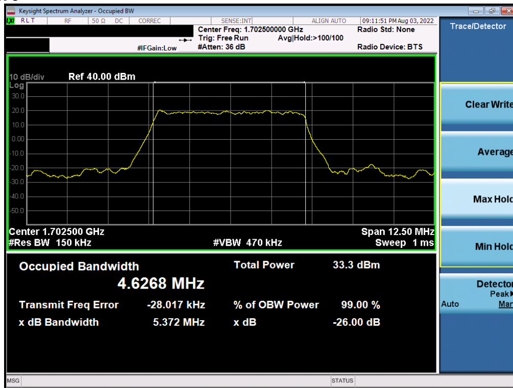
Plot 7-95. Occupied Bandwidth Plot (NR Band n70 - 5.0MHz DFT-s-OFDM \pi/2 BPSK - Full RB)
