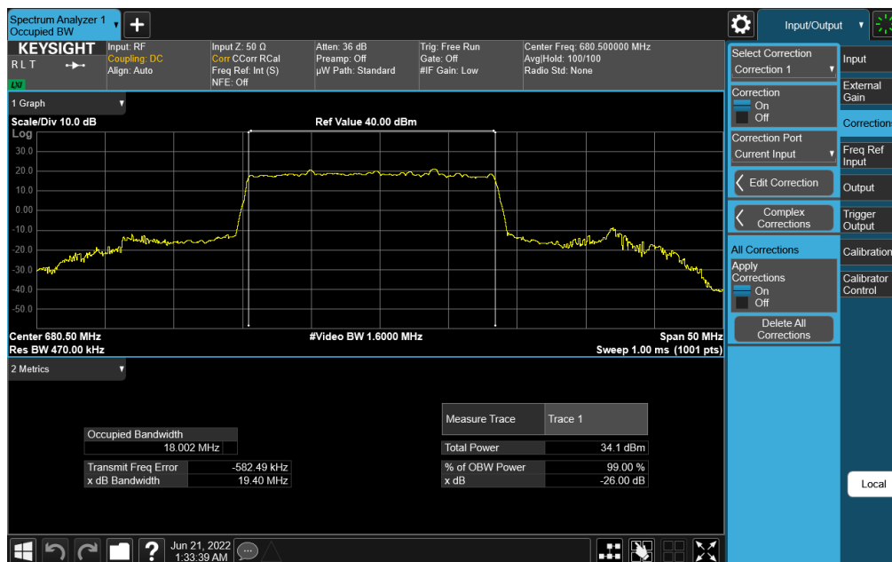
Plot 7-125. Occupied Bandwidth Plot (NR Band n71 - 20MHz DFT-s-OFDM \pi/2 BPSK - Full RB)
