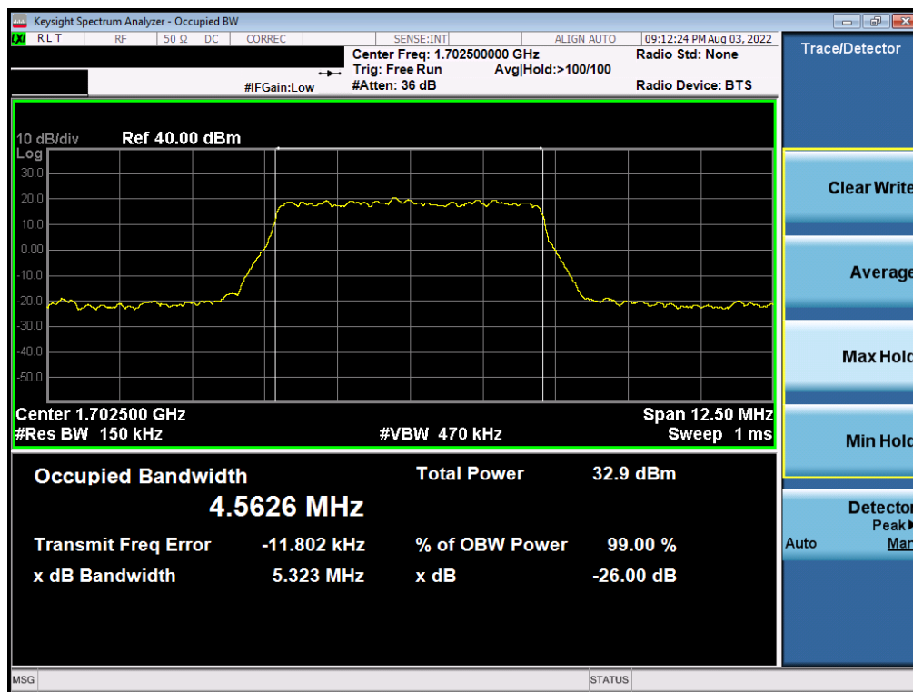
Plot 7-96. Occupied Bandwidth Plot (NR Band n70 - 5.0MHz DFT-s-OFDM QPSK - Full RB)
