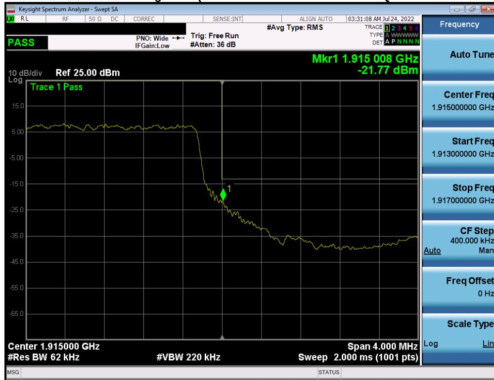
Plot 7-138. Upper Band Edge Plot (NR Band n25 – 5MHz DFT-s-OFDM \pi/2 BPSK – Full RB Configuration)
