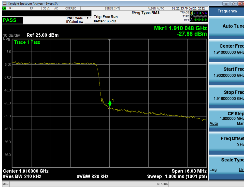
Plot 7-134. Upper Band Edge Plot (LTE Band 2 – 20MHz QPSK – Full RB Configuration)
