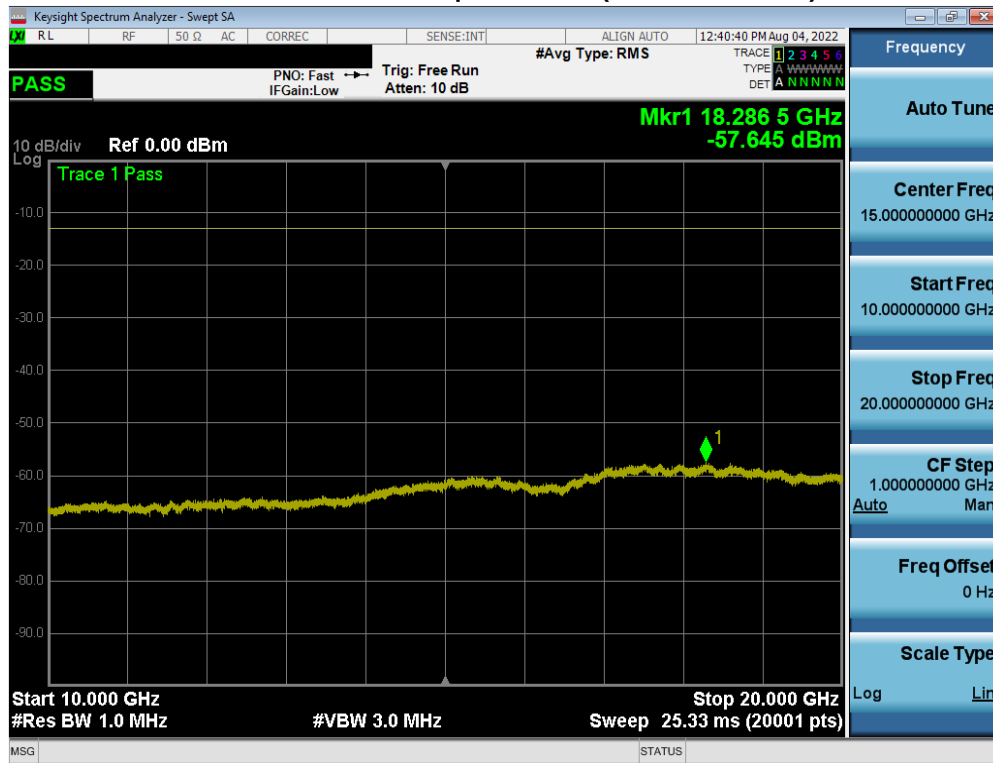
Plot 7-81. Conducted Spurious Plot (WCDMA Ch. 9262)
