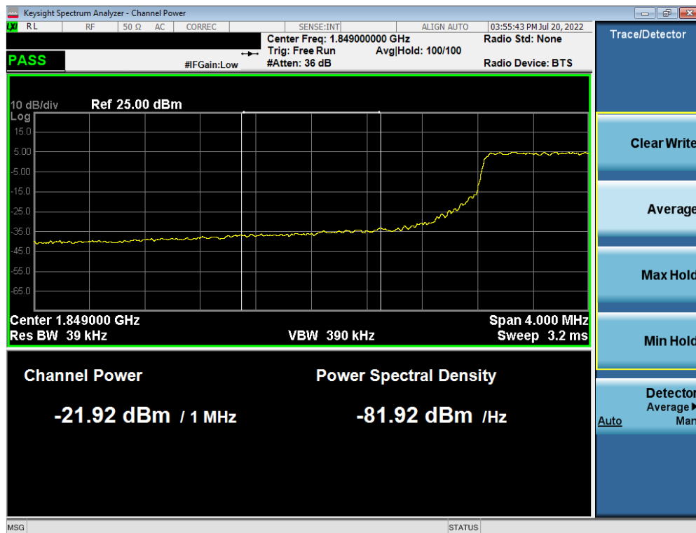
Plot 7-121. Extended Lower Band Edge Plot (LTE Band 2 – 5MHz QPSK – Full RB Configuration)
