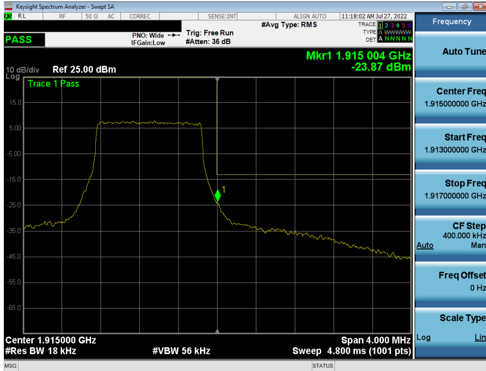
Plot 7-90. Upper Band Edge Plot (LTE Band 25 – 1.4MHz QPSK – Full RB Configuration)
