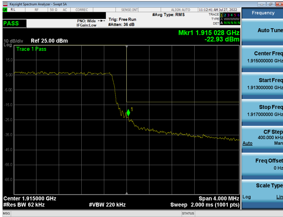
Plot 7-98. Upper Band Edge Plot (LTE Band 25 – 5MHz QPSK – Full RB Configuration)
