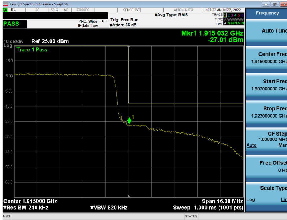
Plot 7-110. Upper Band Edge Plot (LTE Band 25 – 20MHz QPSK – Full RB Configuration)
