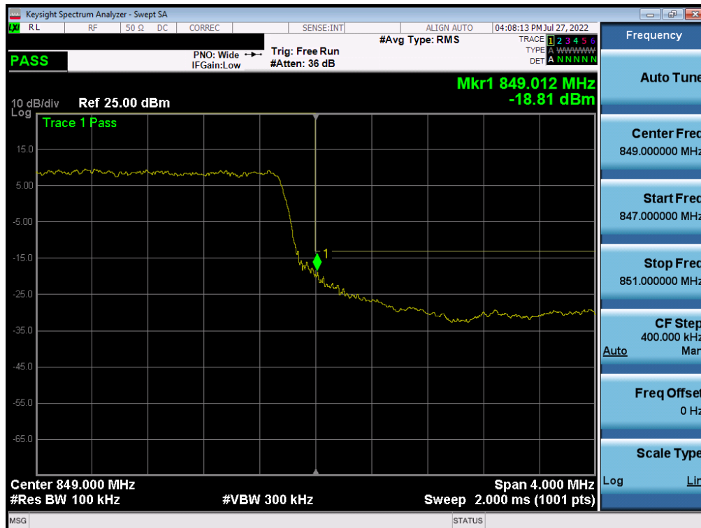
Plot 7-111. Upper BE Plot (NR Band n26 DFT-s-OFDM – 5.0MHz - Full RB)
