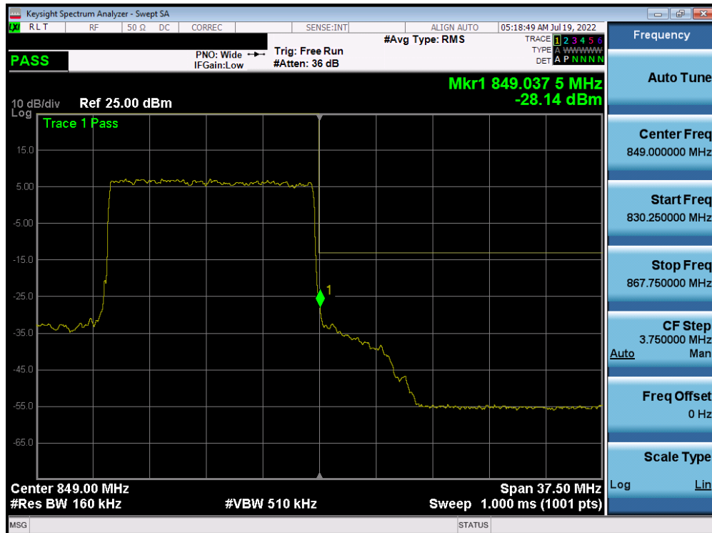
Plot 7-107. Upper BE Plot (NR Band n5 DFT-s-OFDM \pi/2 BPSK – 15.0MHz - Full RB)
