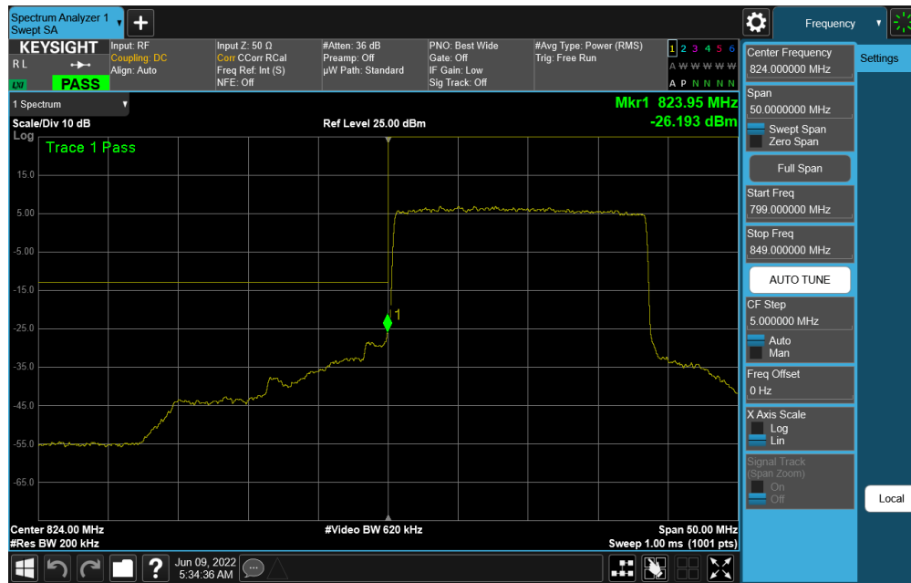
Plot 7-108. Lower BE Plot (NR Band n5 DFT-s-OFDM \pi/2 BPSK – 20.0MHz - Full RB)
