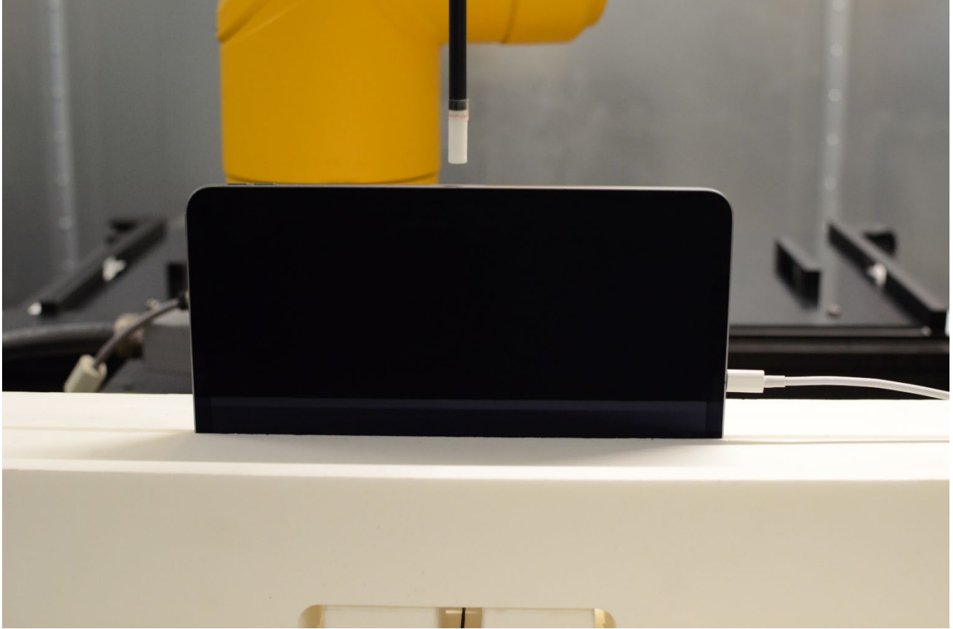
Figure F-10 Near Field Power Density Test Setup Photo – Right Edge at 8.58 mm
