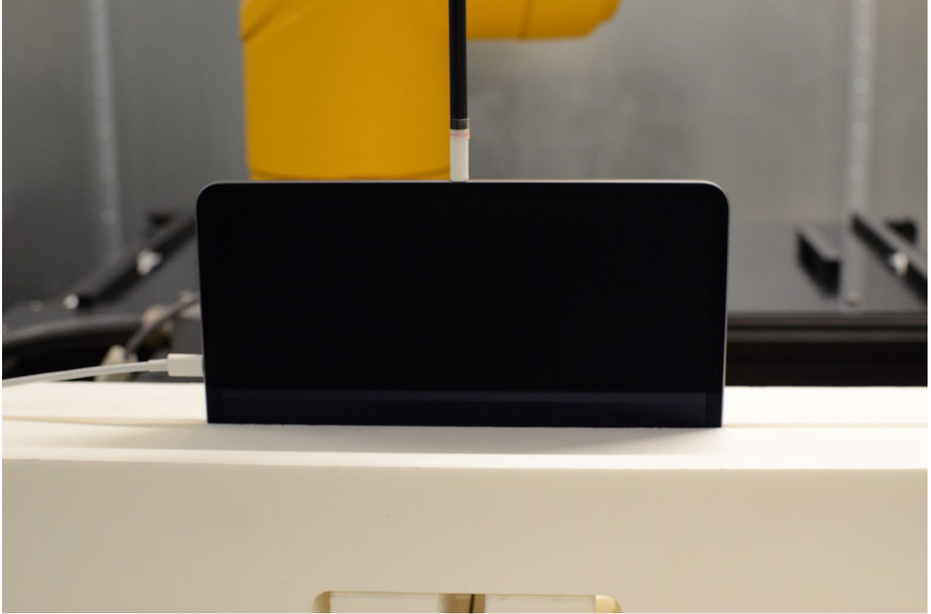
Figure F-11 Near Field Power Density Test Setup Photo – Left Edge at 2 mm
