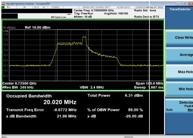
Plot 7-38. 26dB & 99% Bandwidth Plot Antenna WF5t (40MHz 802.11ax RU26 (UNII Band 7) – Ch. 155)
