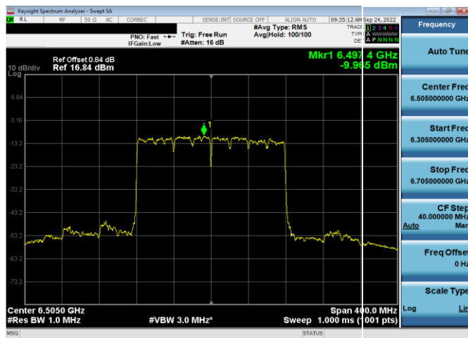
Plot 7-319. Power Spectral Density Plot SDM Antenna WF5t (160MHz 802.11ax (UNII Band 6) – Ch. 111, MCS11)
