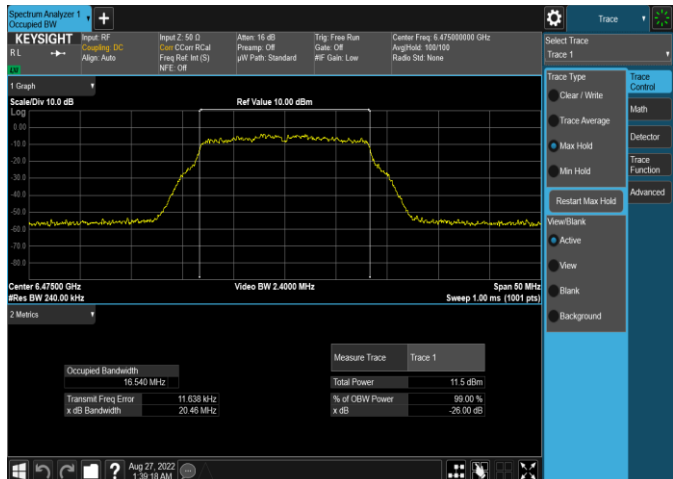
Plot 7-26. 26dB & 99% Bandwidth Plot Antenna WF5t (20MHz 802.11a (UNII Band 6) – Ch. 105, 24Mbps)
