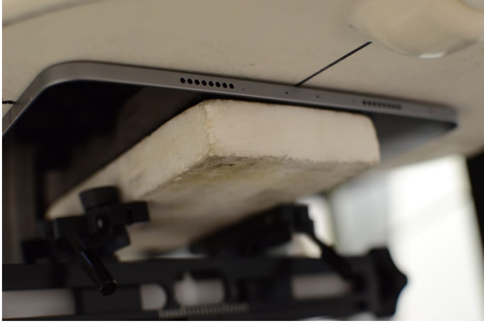
Figure F-3 SAR Test Setup Photo – Back Side at 0 mm
