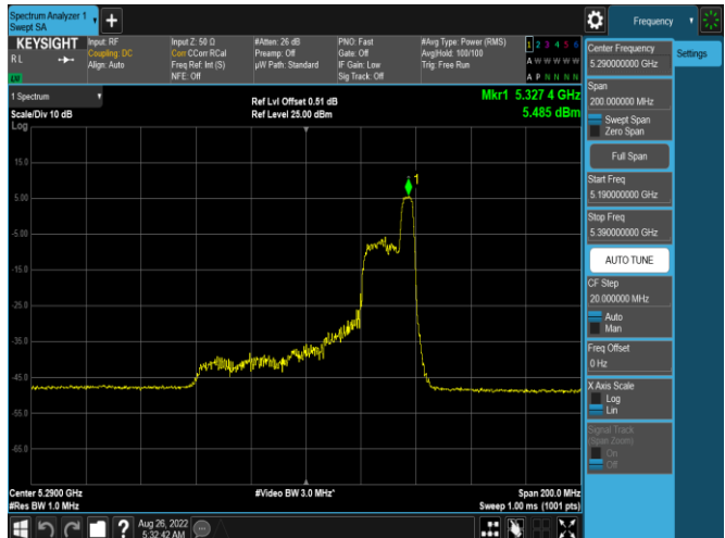
Plot 7-307. PSD CDD Antenna WF5T (80MHz BW 11ax Index 52 - RU52 - Ch.58)
