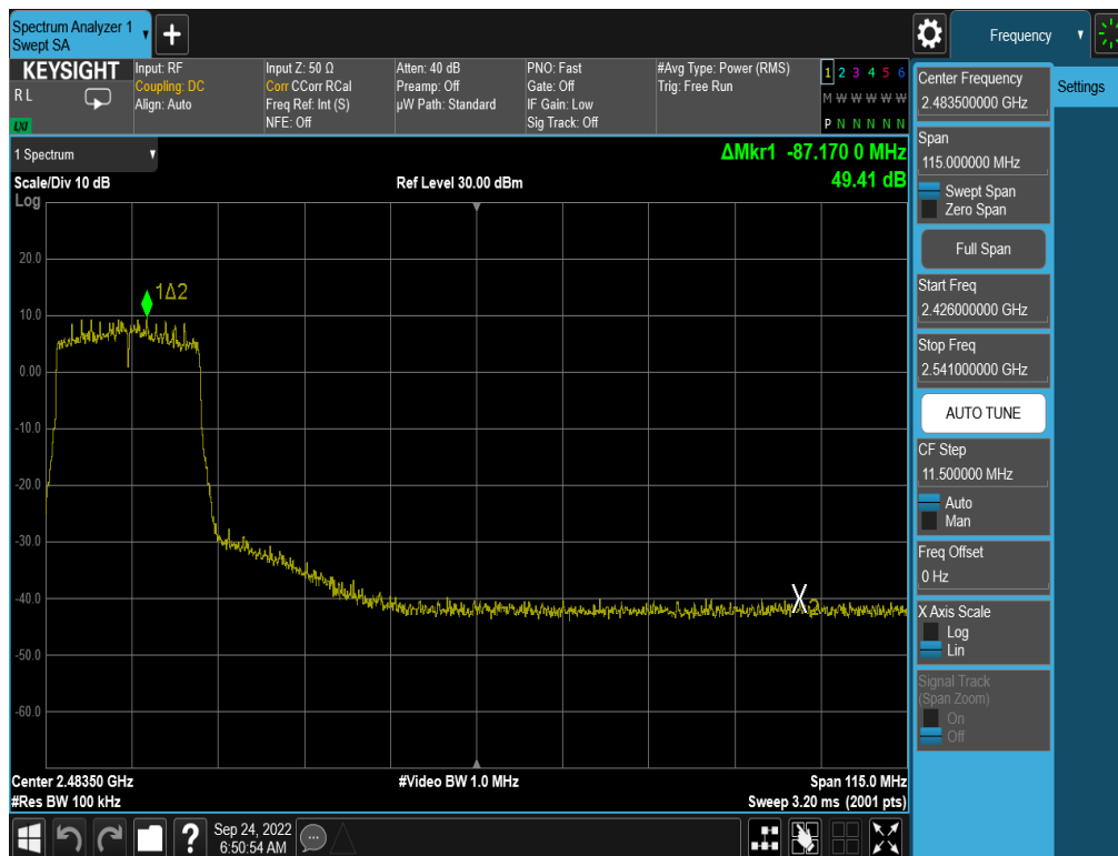
Plot 7-381 . Band Edge Plot Antenna WF7 (802.11ax (SU - 2.4GHz) – Ch. 6 (high)) – MCS3
