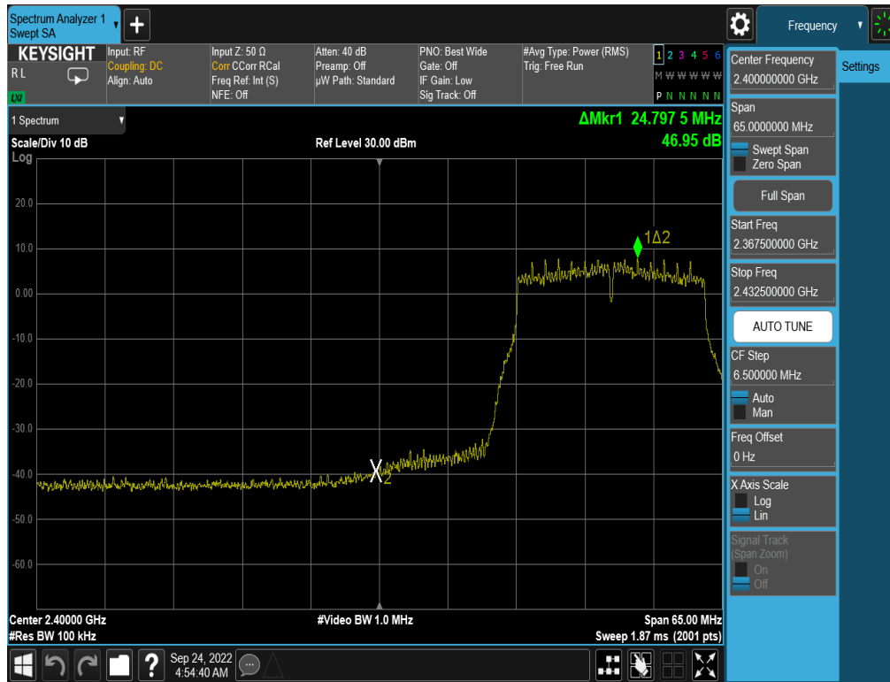
Plot 7-232. Band Edge Plot Antenna WF8 (802.11n (2.4GHz) – Ch. 3) – MCS3
