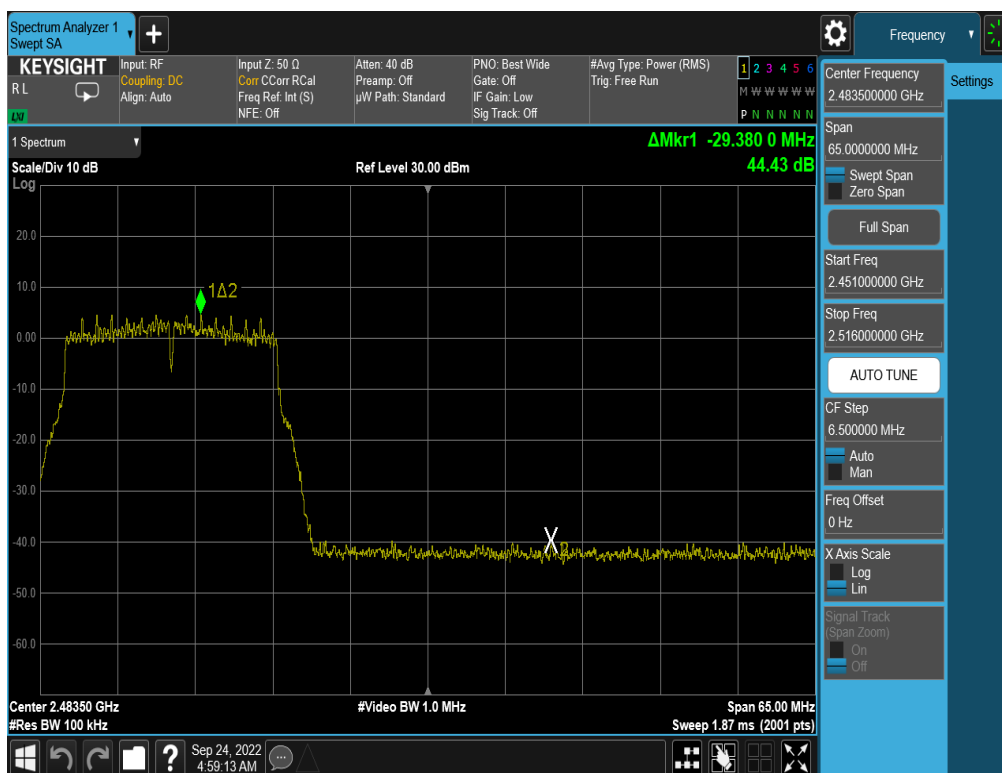
Plot 7-241. Band Edge Plot Antenna WF8 (802.11n (2.4GHz) – Ch. 11) – MCS3
