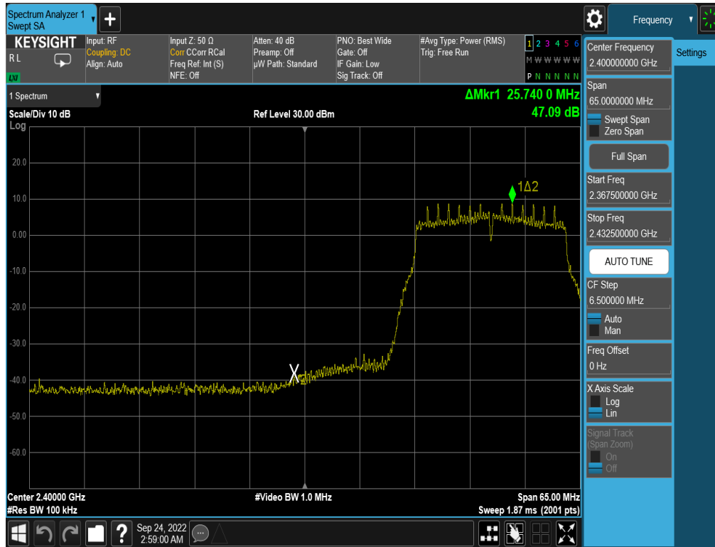
Plot 7-191. Band Edge Plot Antenna WF8 (802.11n (2.4GHz) – Ch. 3) – MCS2
