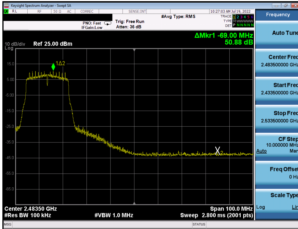
Plot 7-197. Band Edge Plot Antenna WF8 (802.11n (2.4GHz) - Ch. 8) - MCS2
