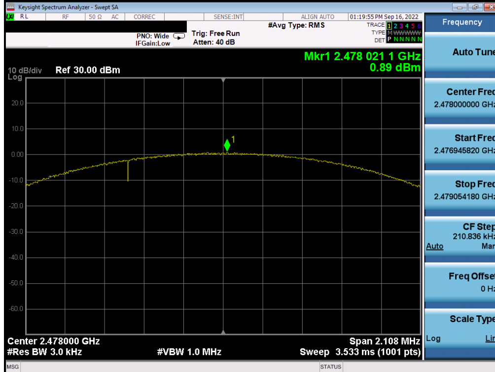
Plot 7-60. Power Spectral Density Plot Antenna WF7 (Bluetooth (LE), 2Mbps, iPA – Ch. 38)
