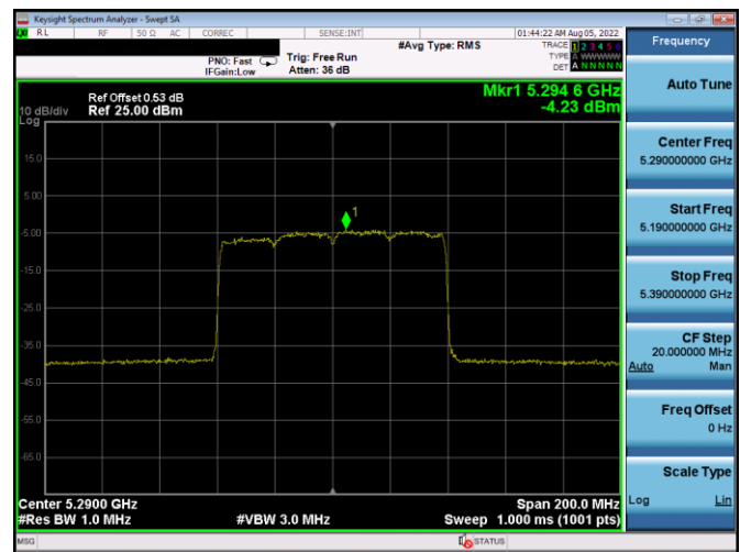
Plot 7-288. PSD Antenna 1b (80MHz BW 11ax - RU996 - Ch.58)
