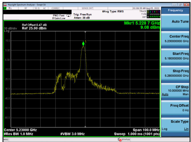
Plot 7-270. PSD Antenna 1b (40MHz BW 11ax Index 8 - RU26 - Ch.46)
