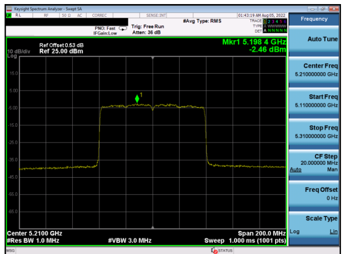
Plot 7-276. PSD Antenna 1b (80MHz BW 11ax – RU996 – Ch.42)
